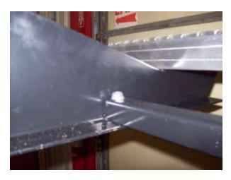
4. Place CB86 between FL501D and FL501P drop 5/16 x 1 1/2" flange bolt through the channel so threads come through the hole in bottom flange of the brackets on each side and put on 5/16 flange nut.
