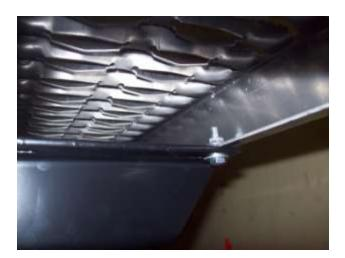
5. Place Aluminum Grip step onto bracket, place a flat washer onto 1/4-20~x~1" bolt, put up through bracket and through hole in bottom lip of the aluminum Grip step tighten the 1/4 flange nut onto each bolt.
