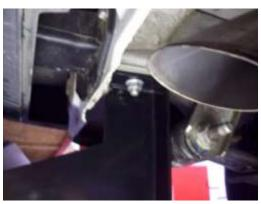
2. On driver side place FL501D up over bolt of the stud plate assembly place 1/2-13 flange nut onto bolt and hand tighten, leave loose for later adjustment.
