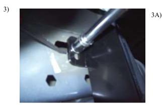
It may be necessary to use a small screw driver to hold against the re-enforcement nut to keep it from turning while tightening the bolt.
