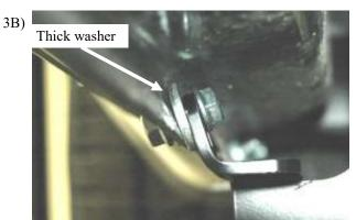
On vehicles produced after July 2015 Chrysler has added a reinforcement bracket on the driver side front location. Install with re-enforcement nut like previously instructed only a thick washer will be placed between bracket and pinch weld as show above.
