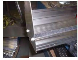
Attach the stone guard and end caps to the board with 3/8" self threading bolts. (extruded board shown)
