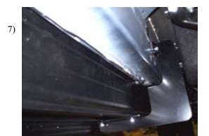
Place the board on the brackets with bolts through slots. Attach with 1/4" nuts loose.
