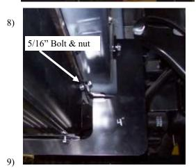
At this time place 5/16" bolt through hole in pinch weld and place nut onto threads. This is done after 1/4" bolts & nut in board are placed into bracket for easier installation of 1/4" bolt into slots of brackets.
