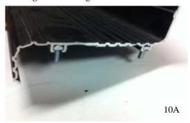
10) Insert Mounting Bolts and Install End Caps **For Aluminum Boards**
