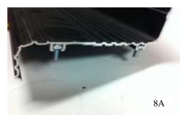
8) <u>Insert Mounting Bolts and Install End Caps</u> <u>For Aluminum Boards</u>
