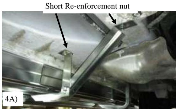
**STEP 4:** Mount a BT70 on the rocker panel using 5/16" x 1-1/2" bolt through washer and BT70 then thread into short re-enforcement nut. Slide nut into hole in lower rocker panel. **When tightening, slide bolt up to edge of hole in body to insure maximum support of the short re-enforcement nut.**
