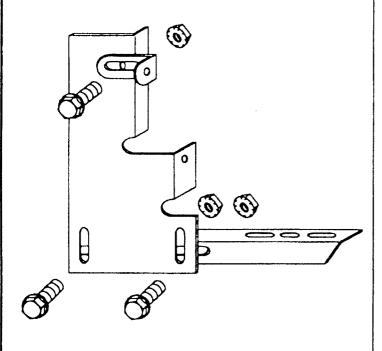
BRACKET ASSEMBLY MOUNT TO BODY ASSEMBLE WITH 5/16 BOLTS AND \$14 SELF DRILLING TEX SCREW
