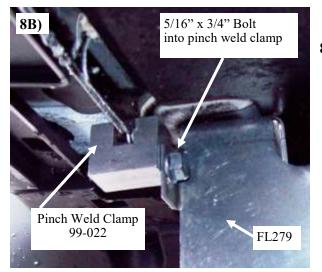
8B) Thread a 5/16" x 3/4" bolt through the slot in FL279 and into pinch weld clamp (99-022) Picture 8B
