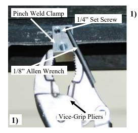
At each mark, mount the pinch weld clamp. You will have to pry the lower plastic away to fit clamp onto pinch weld metal. Tighten the set screws with 1/8" Allen wrench holding with pair of vise grips for leverage.
