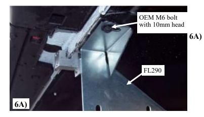
Remove the M6 bolt with 10mm socket. Place bolt through the top slot in FL290 bracket and thread back into threaded hole removed from. **Picture 6A**
