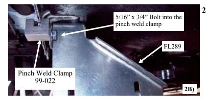
**2B)** Thread a 5/16" x 3/4" bolt through the slot in FL289 and into pinch weld clamp (99-022) **Picture 2B**
