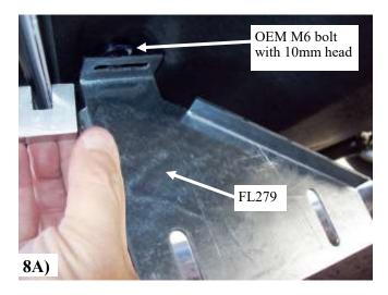
**8A)** Remove the M6 bolt with 10mm socket. Place bolt through the top slot in FL279 bracket and thread back into threaded hole removed from. **Picture 8A**
