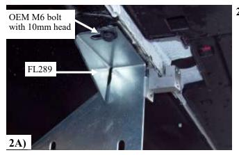
2A) Remove the M6 bolt with 10mm socket. Place bolt through the top slot in FL289 bracket and thread back into threaded hole removed from. **Picture 2A**
