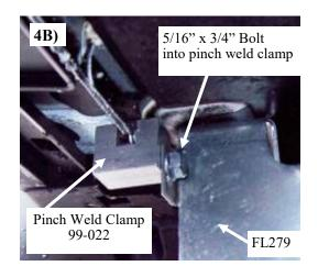
**4B)** Thread a 5/16" x 3/4" bolt through the slot in FL279 and into pinch weld clamp (99-022) **Picture 4B**
