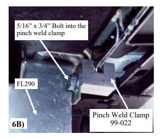
**6B)** The slot on other side of FL290 should like up with the threaded hole in pinch weld clamp (99-022) thread a 5/16" x 3/4" bolt through the slot in FL290 and into pinch weld clamp (99-022) **Picture 6B**
