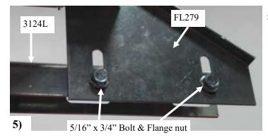
5) Mount the 3124L channel onto FL279 with two 5/16" x 3/4" bolt and flange nuts. **Picture 5**
