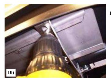
10) Place the running board on the brackets and center board between the front and rear mud flap. Install the self tapping screws through the 3124L bracket and into the galvanized steel plate on the under side of the board.
