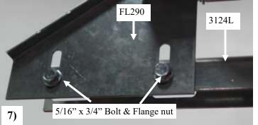
7) Mount the 3124L channel onto FL290 with two 5/16" x 3/4" bolt and flange nuts. **Picture 7**
