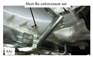
STEP 4: Mount a BT70 on the rocker panel using 5/16" x 1 -1/2" bolt through washer and BT70 then thread into short re-enforcement nut. Slide nut into hole in lower rocker panel. When tightening, slide bolt up to edge of hole in body to insure maximum support of the short re-enforcement nut.
