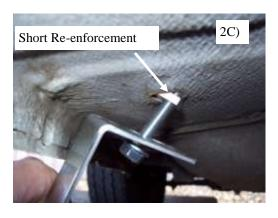
**STEP 2**: At marked bracket locations, remove plastic or rubber plugs in lower rocker panel and frame rail.
