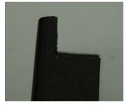
For a Ford Super Duty truck notch top 1" x 1" cutting with diagonal cutter nipping about 1/4" at a time, or cut with saw if available.
