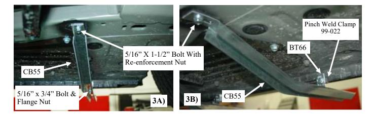
Put a 5/16" x 1-1/2" bolt through the top tab of the CB55 and thread a couple threads into re-enforcement nut. Slide the re-enforcement nut into the hole at 10" in frame rail tighten up tab up to the frame. **Picture 3A** Take a 5/16" x 3/4" bolt through slot in a BT66 thread into the 99-022 pinch weld clamp. **Picture 3B**
