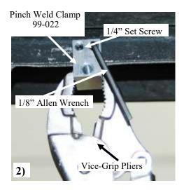
2) At each mark, mount the pinch weld clamp. You have already notched the cladding, put the 99-022 pinch weld clamp onto pinch weld metal. Tighten the set screws with 1/8" Allen wrench holding with pair of vise grips for leverage.
