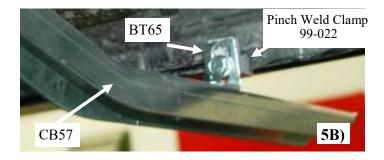
Remove the bolt at 48 1/8" in frame rail with a 13mm socket and place the bolt through the top tab of the CB57 and thread back into hole removed from and tighten CB57 tab up to the frame. **Picture 5A**Take a 5/16" x 3/4" bolt through slot in a BT65 thread into the 99-022 pinch weld clamp. **Picture 5B**
