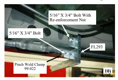
10) Put a 5/16" x 3/4" bolt through the top slot of the FL293 and thread a couple threads into re-enforcement nut. Slide the re-enforcement nut into the hole at 68" in back of the rocker panel. **Picture 10**Take a 5/16" x 3/4" bolt through lower slot in a FL293 thread into the 99-022 pinch weld clamp. **Picture 10**
