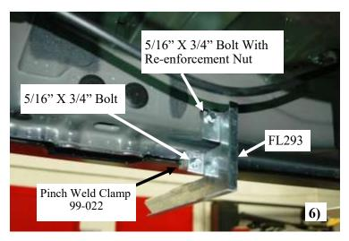
Put a 5/16" x 3/4" bolt through the top slot of the FL293 and thread a couple threads into re-enforcement nut. Slide the re-enforcement nut into the hole at 68" in back of the rocker panel. **Picture 6**Take a 5/16" x 3/4" bolt through lower slot in a FL293 thread into the 99-022 pinch weld clamp. **Picture 6**
