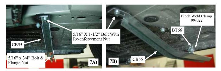
Put a 5/16" x 1-1/2" bolt through the top tab of the CB55 and thread a couple threads into re-enforcement nut. Slide the re-enforcement nut into the hole at 10" in frame rail tighten up tab up to the frame. **Picture 7A** Take a 5/16" x 3/4" bolt through slot in a BT66 thread into the 99-022 pinch weld clamp. **Picture 7B**
