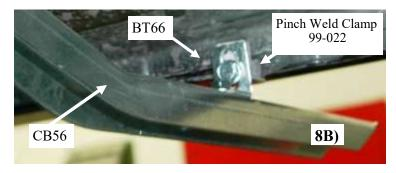
Remove the bolt at 21" in frame rail with a 13mm socket and place the bolt through the top tab of the CB56 and thread back into hole removed from and tighten CB56 tab up to the frame. **Picture 8A**Take a 5/16" x 3/4" bolt through slot in a BT66 thread into the 99-022 pinch weld clamp. **Picture 8B**
