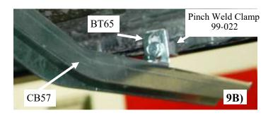
9) Remove the bolt at 48 1/8" in frame rail with a 13mm socket and place the bolt through the top tab of the CB57 and thread back into hole removed from and tighten CB57 tab up to the frame. **Picture 9A**Take a 5/16" x 3/4" bolt through slot in a BT65 thread into the 99-022 pinch weld clamp. **Picture 9B**
