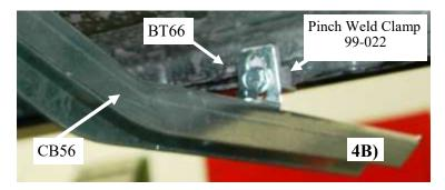
4) Remove the bolt at 21" in frame rail with a 13mm socket and place the bolt through the top tab of the CB56 and thread back into hole removed from and tighten CB56 tab up to the frame. **Picture 4A**Take a 5/16" x 3/4" bolt through slot in a BT66 thread into the 99-022 pinch weld clamp. **Picture 4B**
