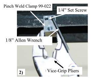
2) At each mark, mount the pinch weld clamp 99-022. You will have to pry the lower plastic away to fit clamp onto pinch weld metal. Tighten the set screws with 1/8" Allen wrench holding with pair of vise grips for leverage.
