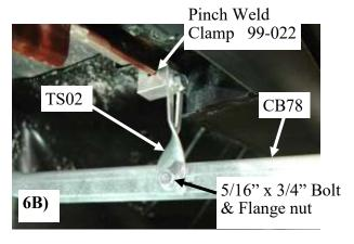
Remove the front OEM bolts with a 12mm socket, place the bolt through the top slots on the CB78 bracket and thread back into the holes that they were remove from. Snug up bolt so bracket is up against the bottom of the frame. Picture 6A
