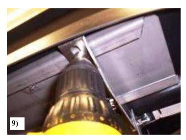
9) Place the running board on the brackets and center board between the front and rear wheel well. Install the self tapping screws through the CB 78 channel brackets on the front and CB88 on rear position and the 3124J bracket on the middle position and into the galvanized steel plate on the under side of the board.
