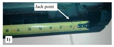
1) Measuring from the front of the jack point as shown in photo. Mark the inside of pinch weld with a marker.
