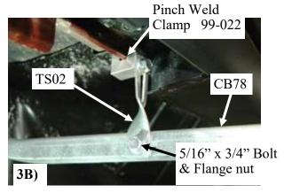
Remove the front OEM bolts with a 12mm socket, place the bolt through the top slots on the CB78 bracket and thread back into the holes that they were remove from. Snug up bolt so bracket is up against the bottom of the frame. **Picture 3A**
