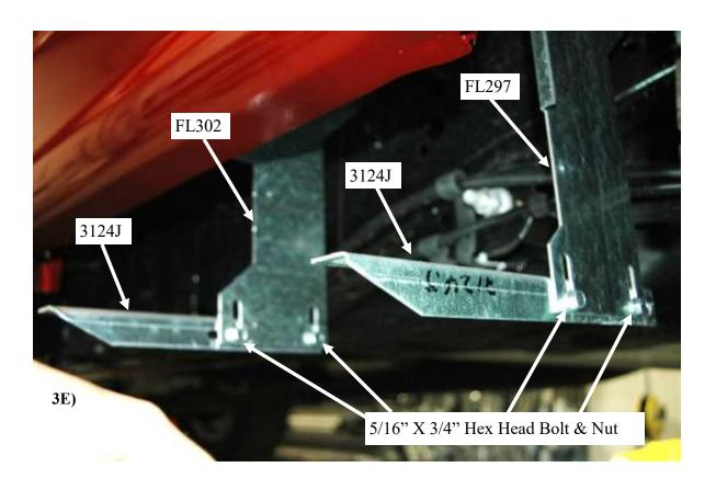
Place the 3124J angle bracket onto the FL302 and FL297 brackets and secure to each other with two 5/16" x 3/4" hex head bolts and two flange nuts. **Picture 3E**
