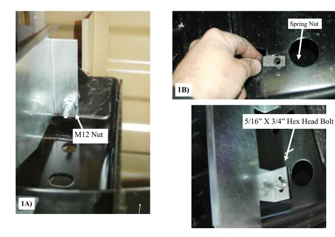
On the front bed rail locate the bolt holding the bed to frame, slide the FL 302 rear slot onto the threads coming through the frame. Thread a M12 onto the threads to secure FL302. Slide a 5/16" spring clip into slot in frame and place a 5/16" x 3/4" flange bolt through the hole in tab coming off the FL302 bracket
