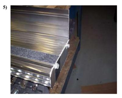
Attach stone guard and end cap to running board using 3/8"self threading bolts.
