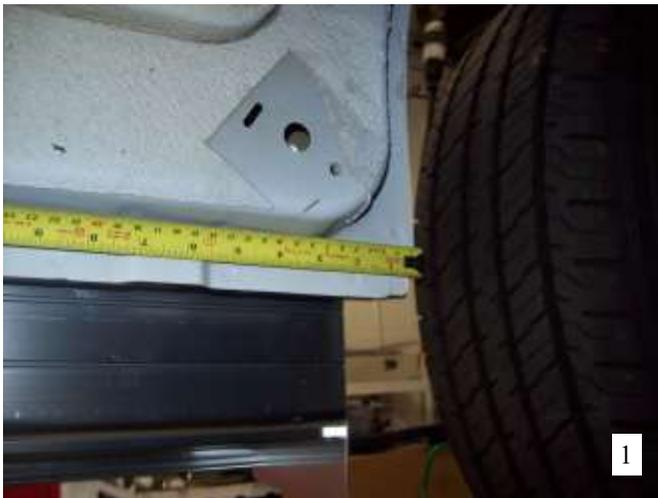
Measuring from the front wheel well back, **Fig 1** mark the following locations on the pinch weld. There will be factory holes in line with these marks that will be used to mount the running board brackets
