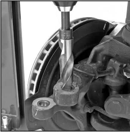
1) After removing the stock tie rod & drag link, if you are using the reversed drag link kit, drill the drag link taper out with a 7/8" drill bit.
