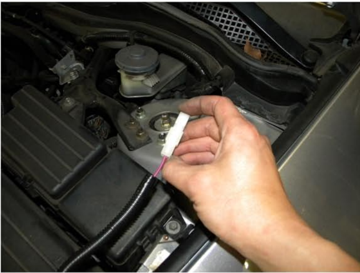
41. Connect the extension wire to the switch power wire
