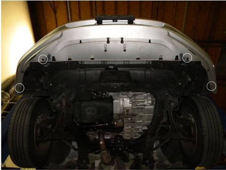
1. (4) 10mm bolts location
