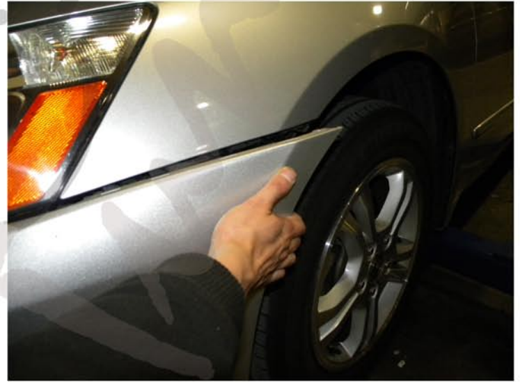
8. Tug on the sides of the front bumper
