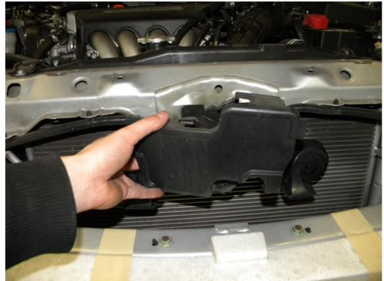
22. Remove the hood latch cover
