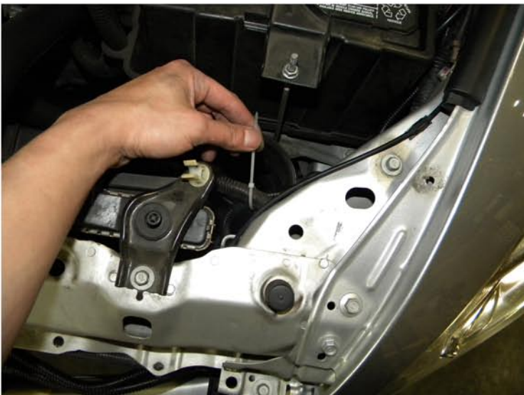
45. Zip the switch power extension wire onto the factory wire harness
