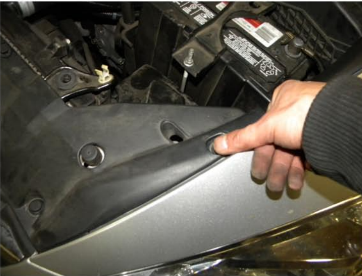
49. Replace the (10) plastic clips
