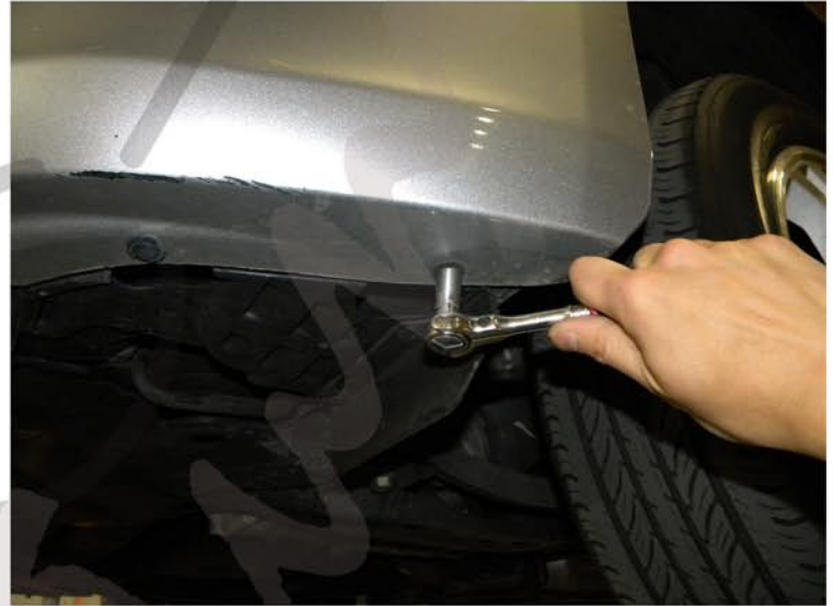
2. Remove the (4) 10mm bolts
