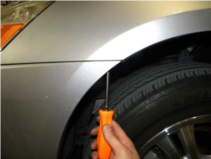
7. Remove the phillips head screw
