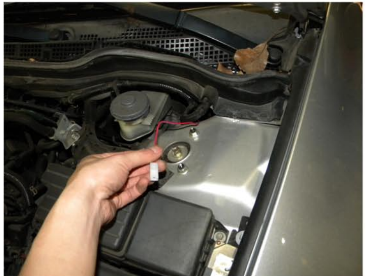
40. Pull the fog light switch power wire through the rubber grommet
