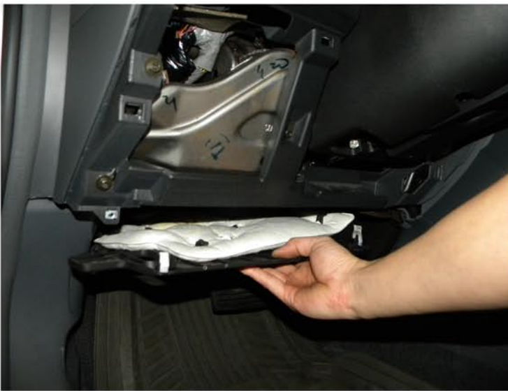
29. Remove the dashboard under cover
