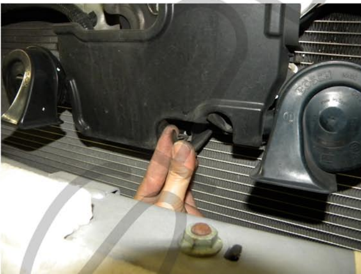
21. Remove the plastic clip
