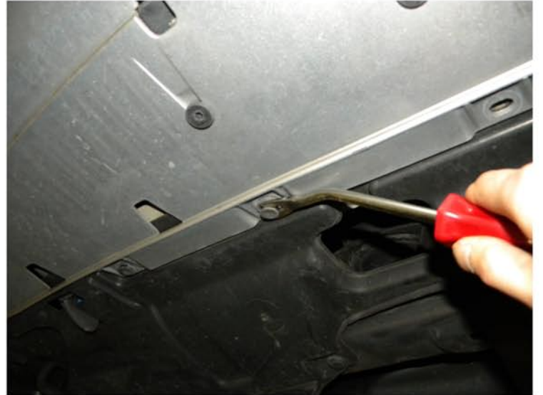
4. Remove the (6) plastic clips
