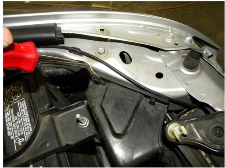
42. Remove the (2) plastic clips
