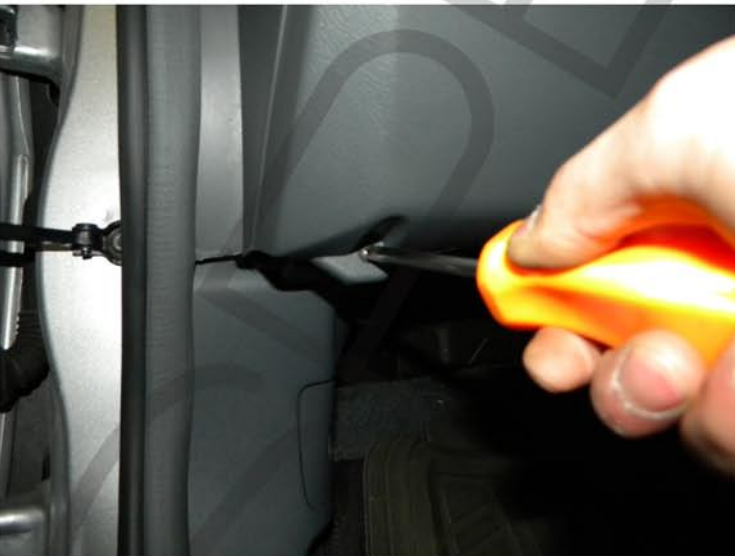
27. Remove the phillips head screw
