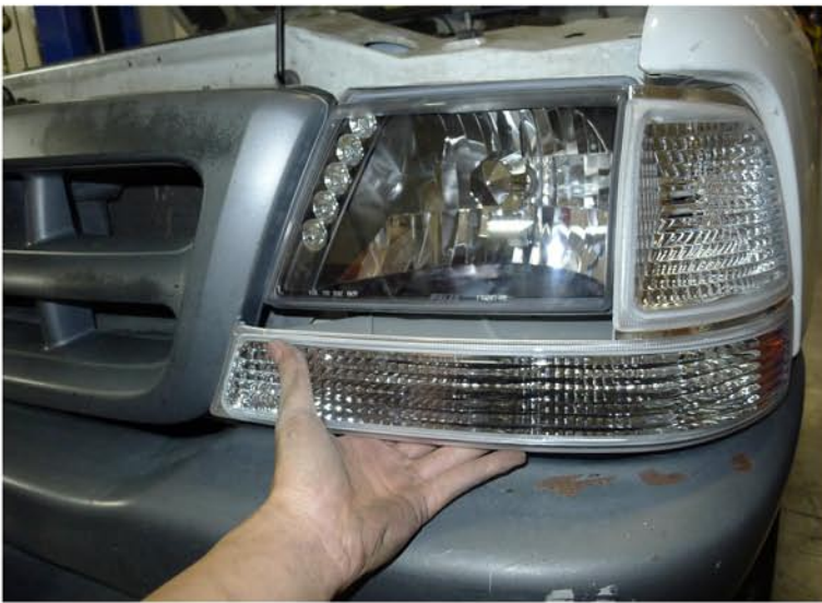
17. Replace the corner bumper light
