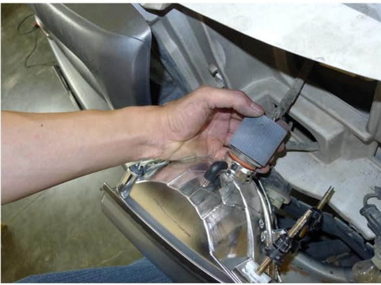
11. Install the headlight bulb into the new headlight
