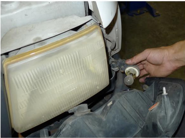
5. Disconnect the light sockets
