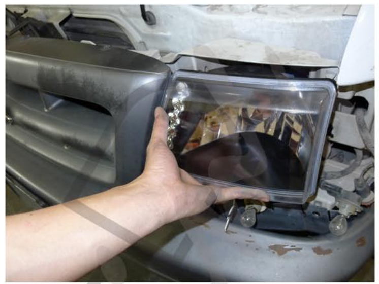
12. Place the new headlight in the stock location
