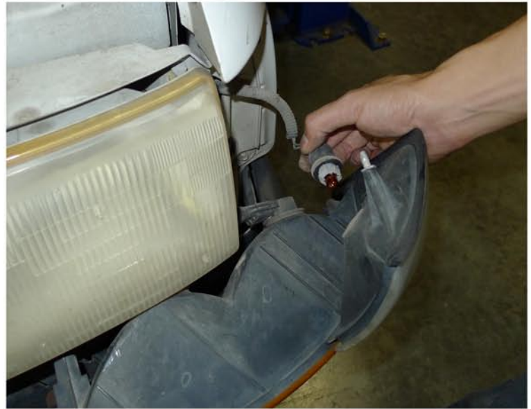
4. Disconnect the light sockets
