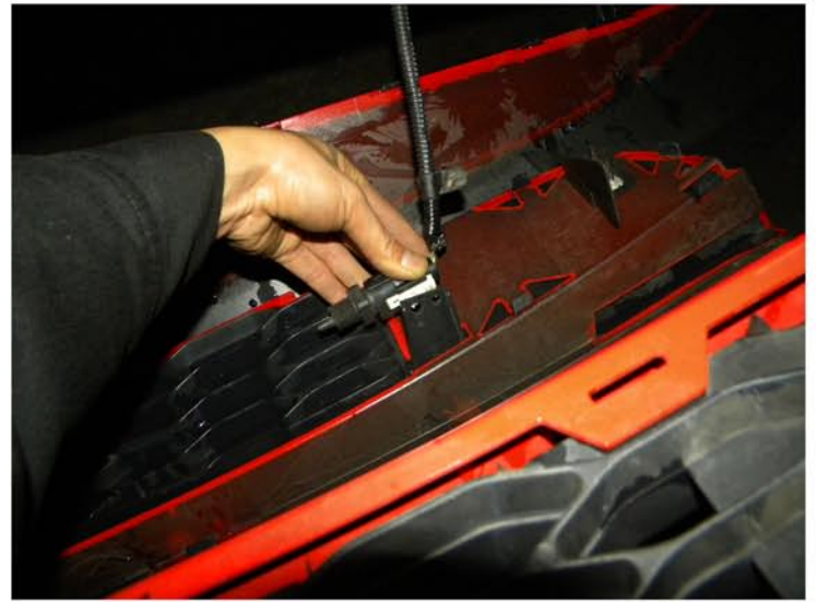
10. Remove the temp sensor from the bracket on the inner side of the bumper
