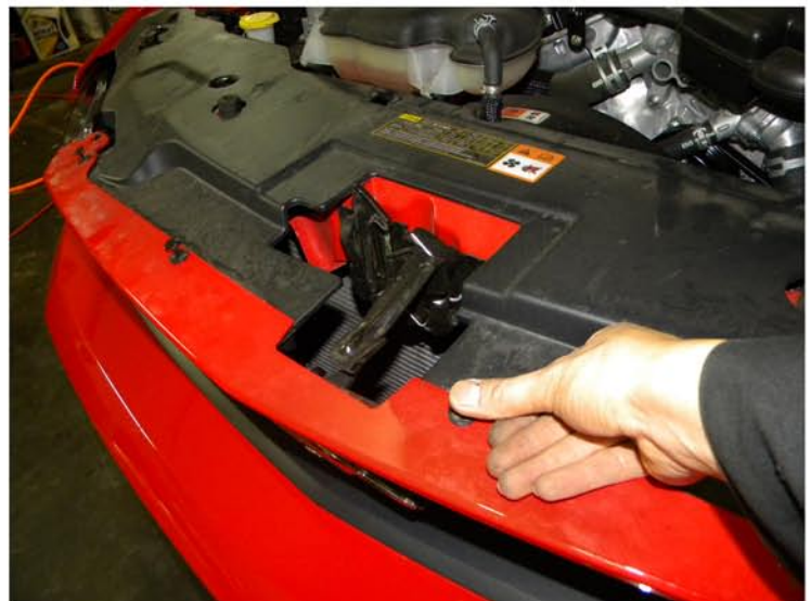
28. Replace the (4) plastic clips on the top side of the front bumper
