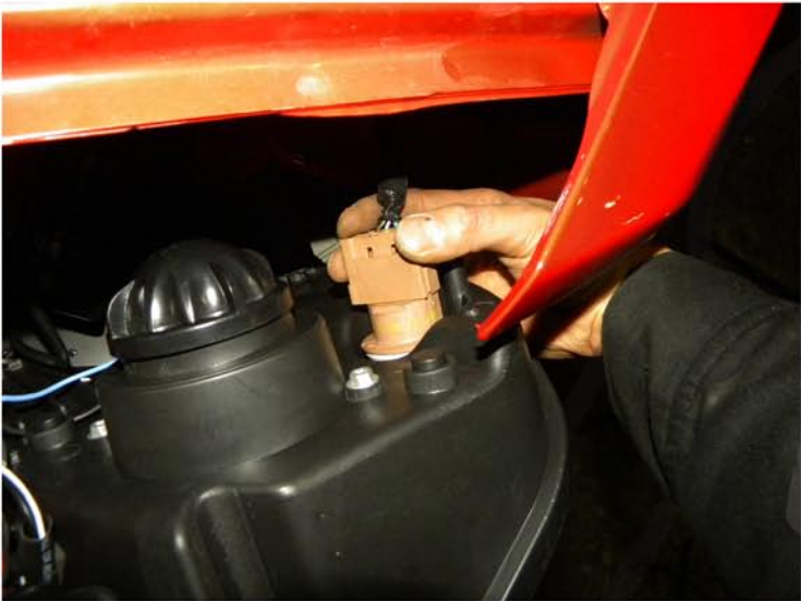
19. Plug the driving light into the new headlight Please see the "Halo and L.E.D installation instructions" If your headlights don't have HALO or L.E.D. You can skip this step
