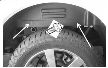
**8.** Re-install the screw saved in step 2; Then tighten the loosen screw from step 3
