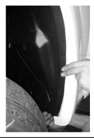
**6.** Insert the upper section of the plastic liner behind the metal flange.
