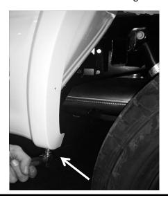
**2.** Locate the 2 holes at the back area of the wheel house and insert one J clip in each hole.
