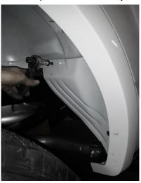
**2.** to avoid interference and facilitate the installation: Locate the screw on the bottom front area of the fender flair; then loosen the screw half the length.
