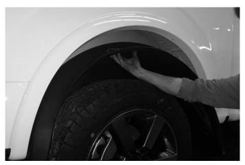
5. Insert the bottom sides behind the metal flange
