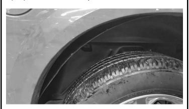
**3.** Insert the bottom sides behind the metal flange.
