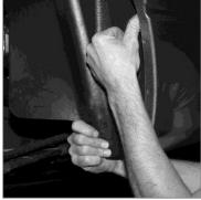
**4.** Insert the upper section of the plastic liner behind the metal flange, make sure all the edges are inside the metal wheel well house edge.
