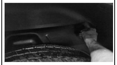
**6.** Locate pre-drilled holes on the body of the Inner Wheel Well Liner, align holes with pre-drilled holes located at the wheel house flange, then install one push lock pin in each hole.
