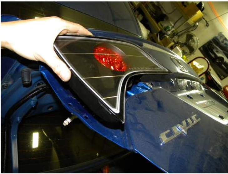
29. Place the tail light in the stock location
