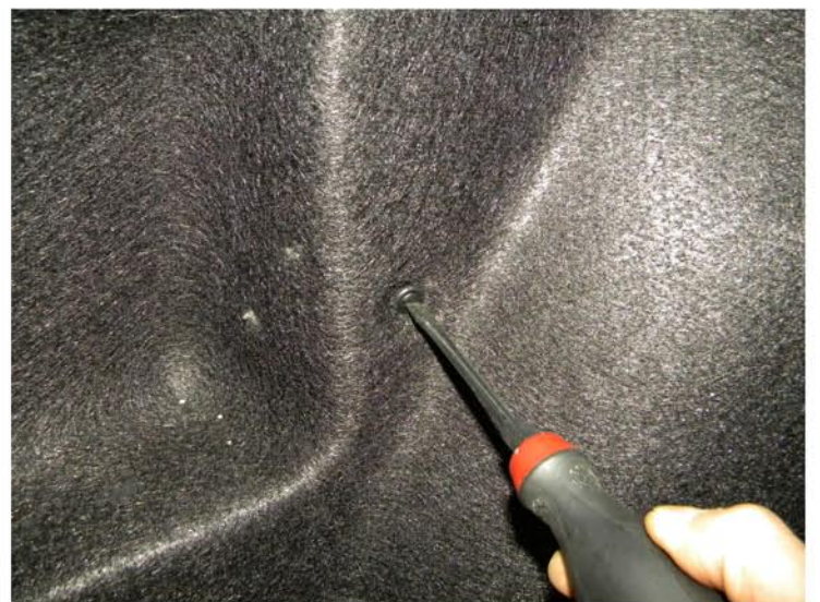
10. Remove the (3) plastic clips
