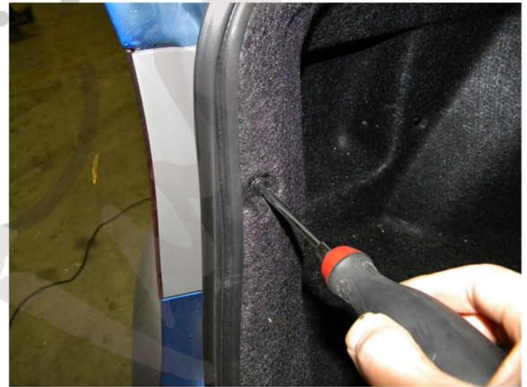
8. Remove the (3) plastic clips
