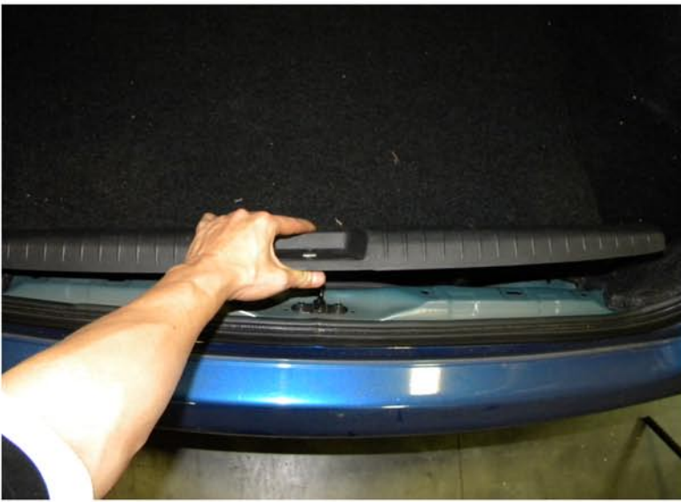
35. Replace the plastic moulding
