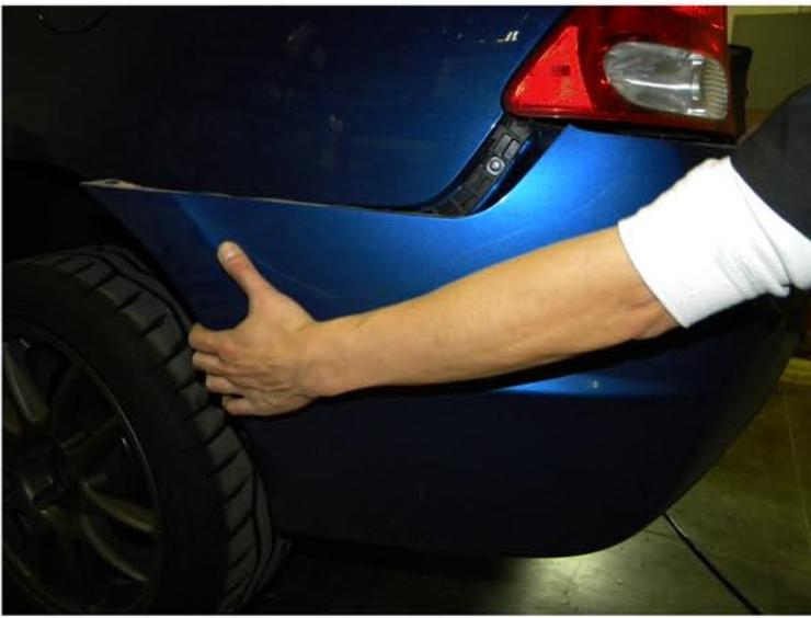
5. Pull the bumper away from the body of the car
