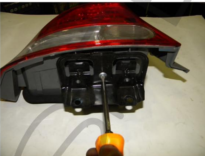
15. Remove the phillips head screw
