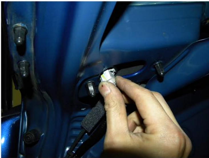
31. Place the harness into the new tail light
