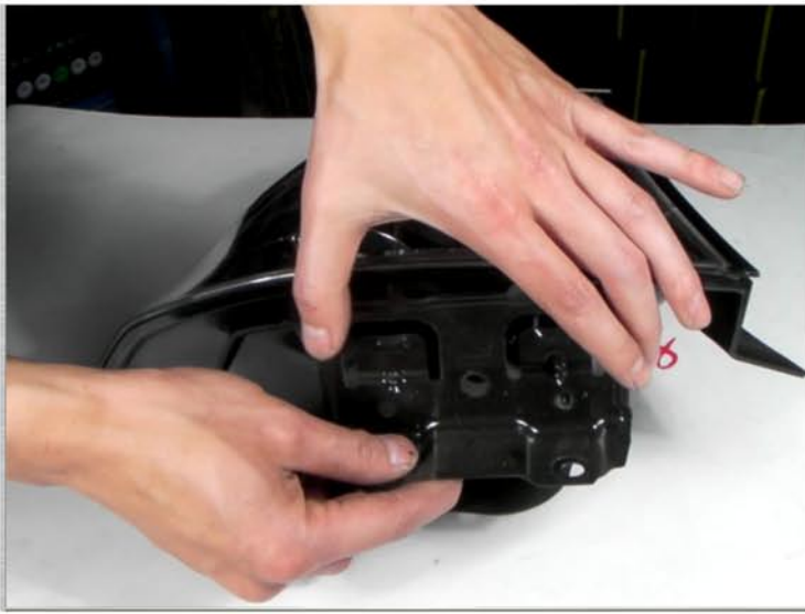
17. Place the bracket on the new light
