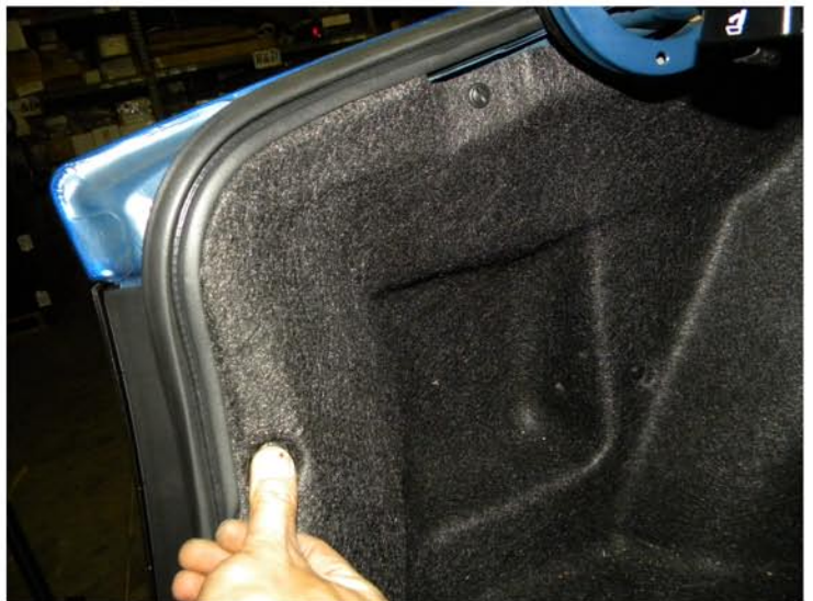
34. Replace the (3) plastic clips
