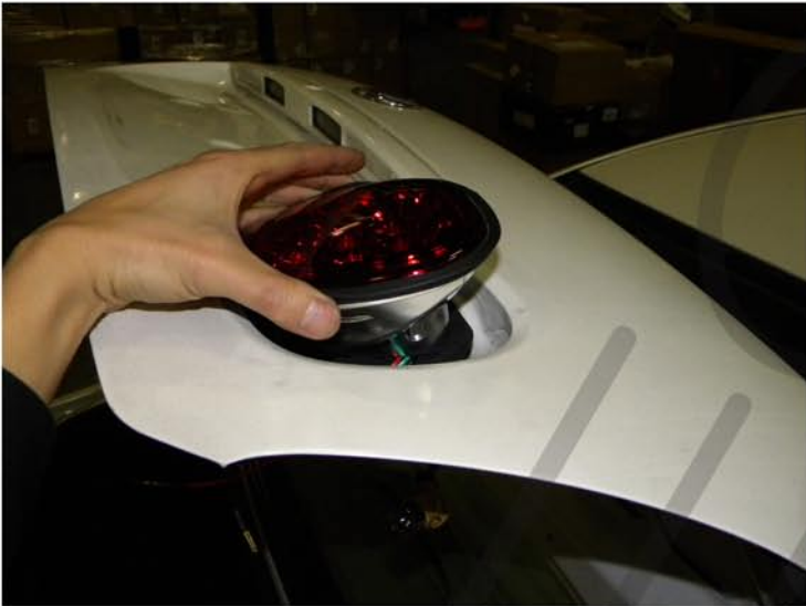
19. Place the LED tail light in the stock location
