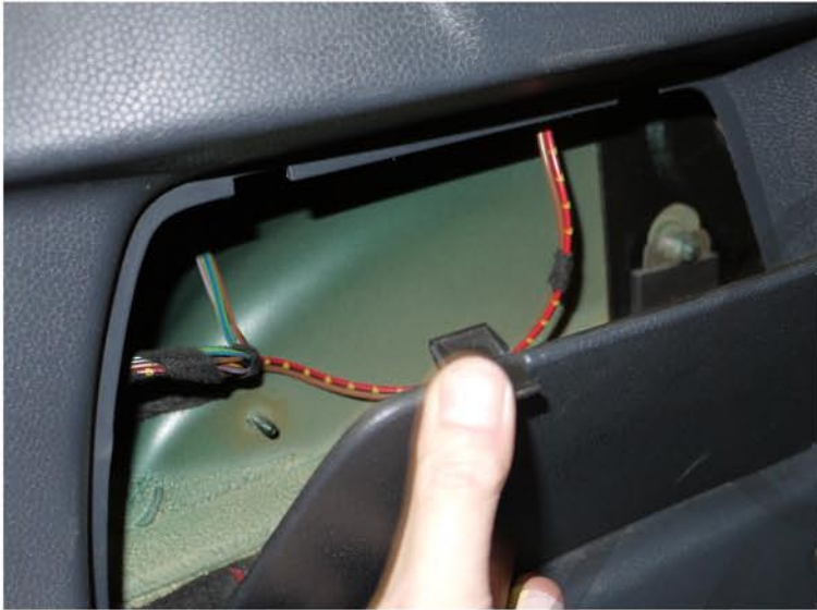
1. Remove the access panel
