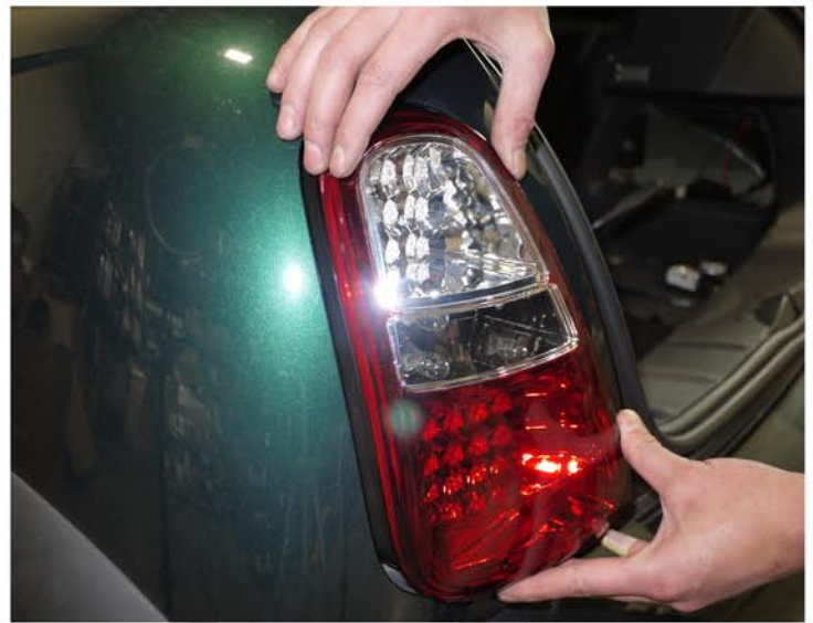
6. Place the LED taillight in the factory location
