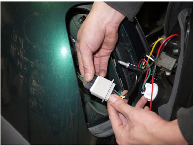
5. Connect the taillight harness to the LED taillight please see the " L.E.D. tail lights installation instructions" If your tail lights don't have L.E.D. you can skip the installation instructions.
