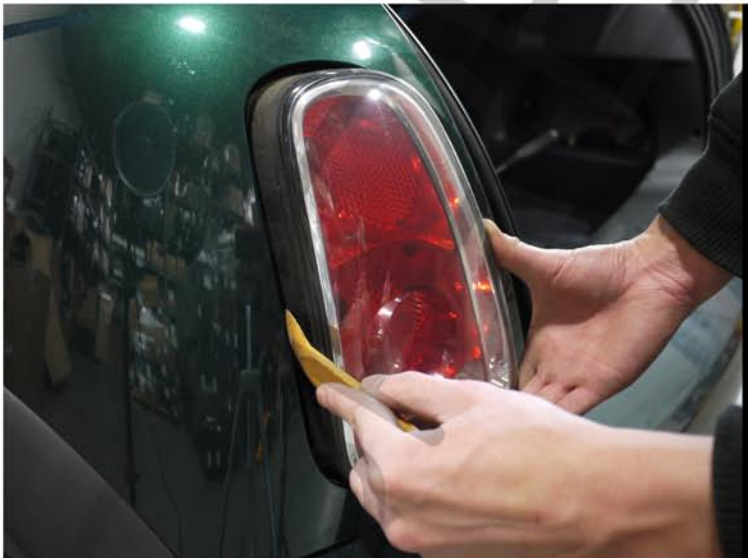
3. Remove the factory taillight
