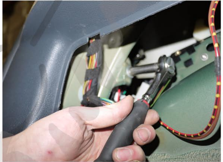
2. Remove the 10mm nut
