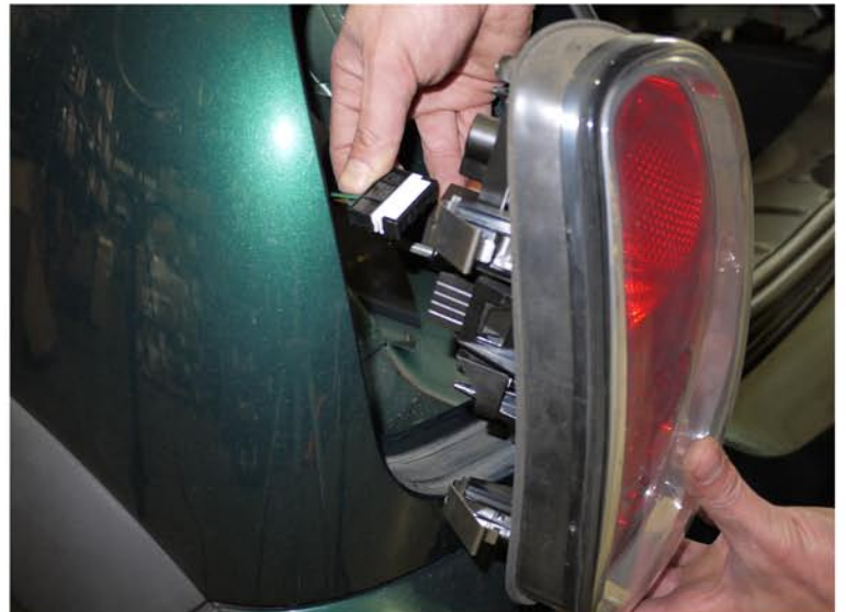
4. Disconnect the factory taillight
