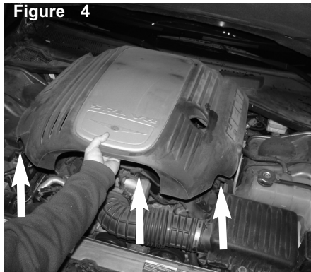
Lift up and remove engine cover.
