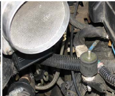
Screw the vibra-mount into the stud until it sits flush and firm.
