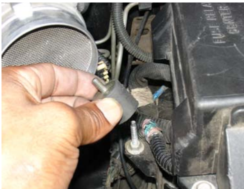
Take the female vibra-mount and screw the female end into the air box m6 stud as shown above.
