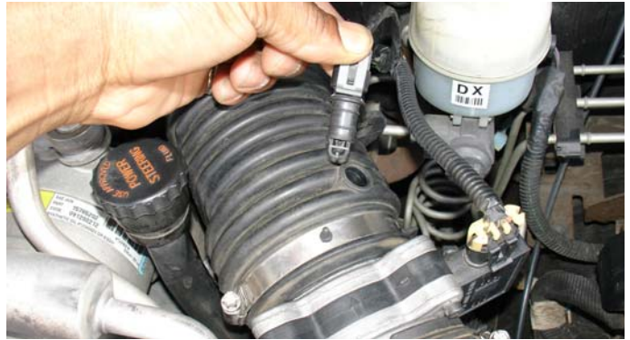
Air temperature sensor is removed from the air intake duct.
