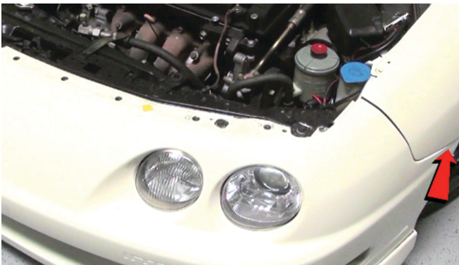
7) Remove [1x] phillips screw securing the fascia in the wheel well on each side.
