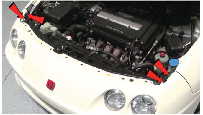
6) Remove [4x] 10mm bolts securing the fascia.
