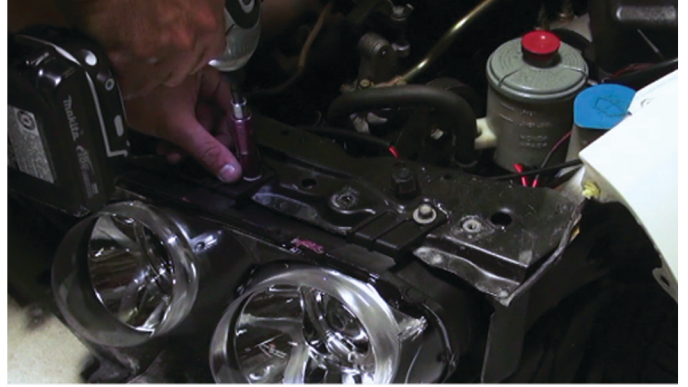
18) Reinstall [4x] 10mm bolts to secure the headlight.
