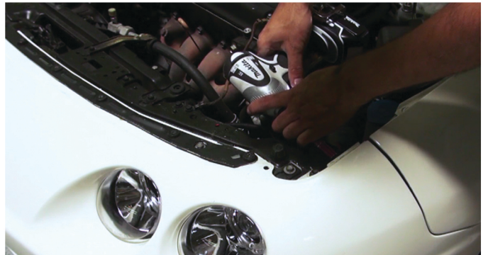
22) Reinstall [4x] 10mm bolts to secure the fascia; [2x] at each upper corner of the fascia.
