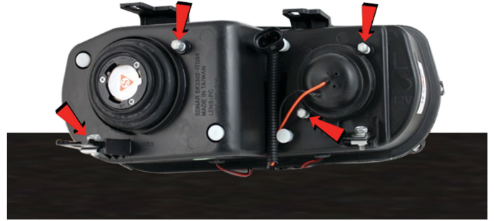
14) The beam adjusters are 8mm and are shown here. See "How To Wire Halos" on the Spyder FAQs Playlist on the Spyder Auto YouTube channel for more information.
