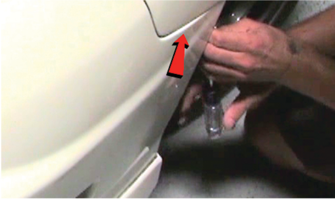
23) Reinstall [1x] phillips screw securing the fascia at the wheel well on each side.
