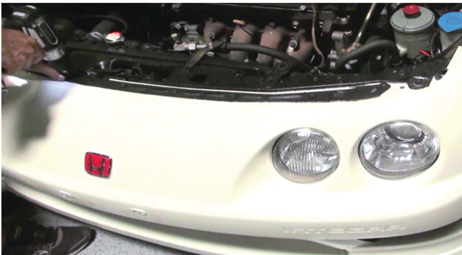
21) Reinstall [9x] Phillips screws to secure the support bracket.
