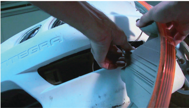
25) Reinstall [2x] turn signal sockets into the corner lamp.
