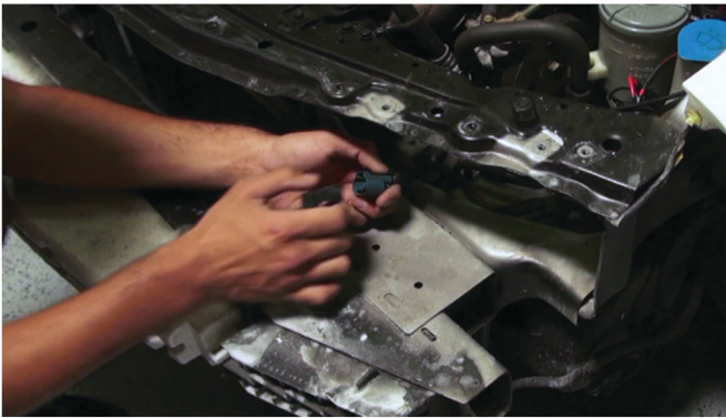
13) Remove the high beam bulb from its socket.
