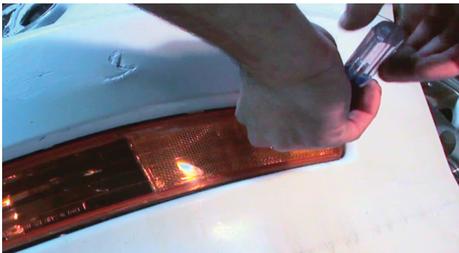
27) Reinstall [1x] phillips screw to secure the corner lamp.
