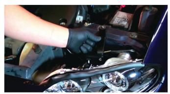
10) Replace the headlight bracket and reinstall [2x] 10mm bolts to secure the bracket.
