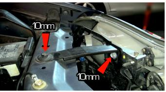
2) Remove [2x] 10mm bolts securing the headlight bracket.
