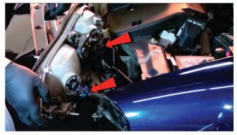
5) Disconnect the high and low beam wiring harnesses, then remove the OEM headlight.
