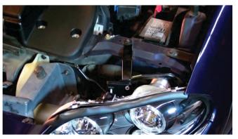
11) Reinstall [2x] 10mm bolts to secure the headlight bracket.
