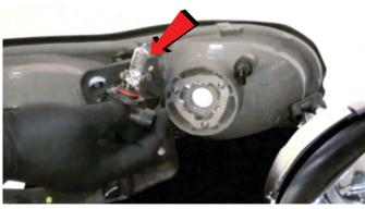
6) Remove the high beam bulb from your OEM headlight. Never touch exposed bulbs with bare hands.
