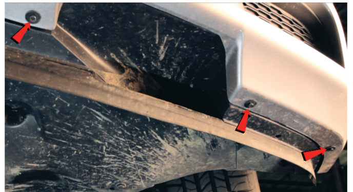
8) Remove [3x] 7mm bolts securing the fascia from below.
