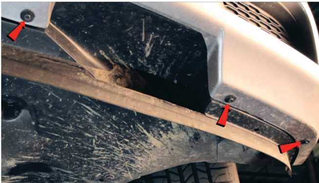
31) Reinstall [3x] 7mm bolts to secure the fascia.
