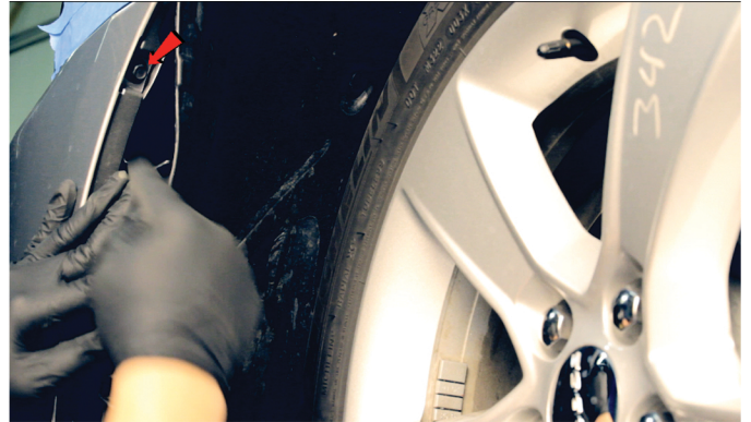
6) Remove [1x] 10mm Bolt securing the fascia.
