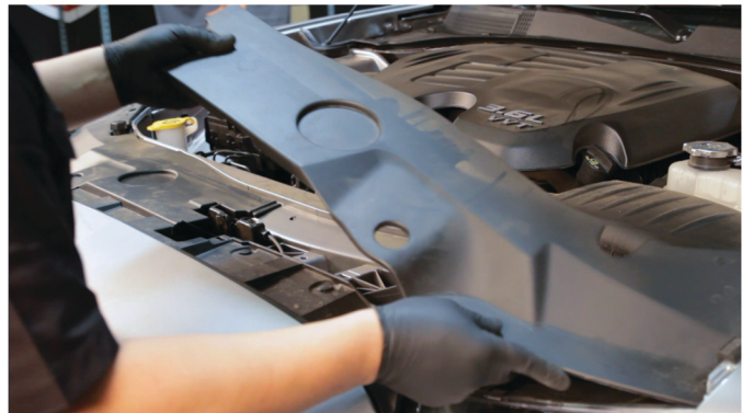
26) Reinstall [2x] filler panels.
