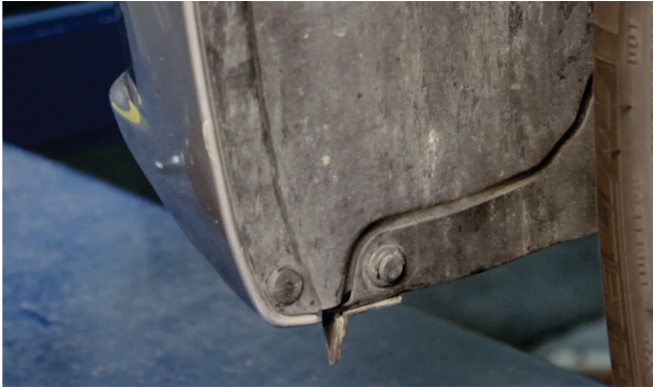
29) Reinstall [2x] plastic retainers to secure the fender liner.
