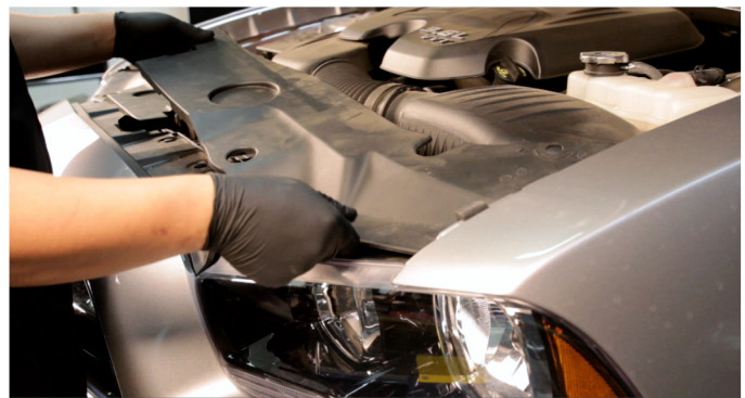
2) Pull up to remove [2x] radiator filler panels. Each filler panel is secured by [5x] clips.
