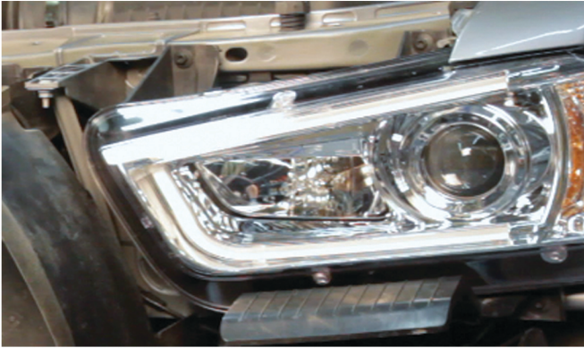
23) Reinstall [4x] 8mm bolts to secure the headlight.
