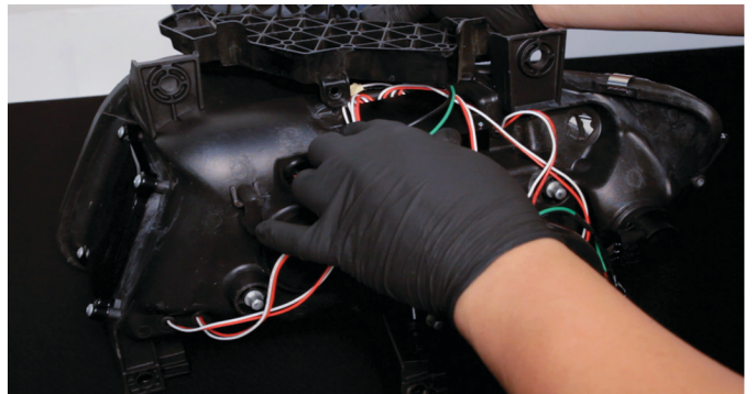
16) Transfer the bumper bracket to the Spyder headlight.
