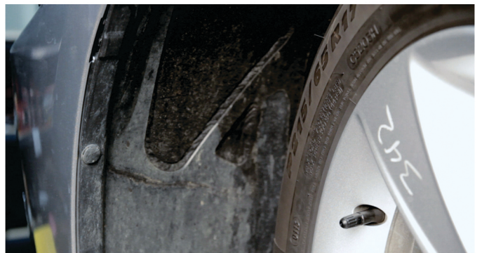
28) Reinstall [1x] plastic retainer to secure the fender liner.
