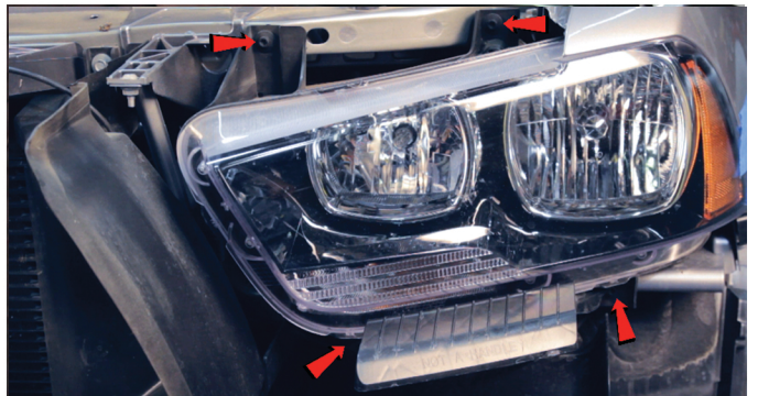
10) Remove [4x] 8mm bolts securing the headlight.
