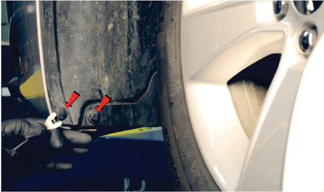
5) Remove [2x] additional plastic retainers securing the fender liner.
