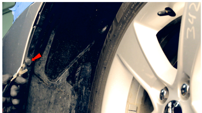
4) Remove the plastic retainer securing the fender liner in the wheel well.
