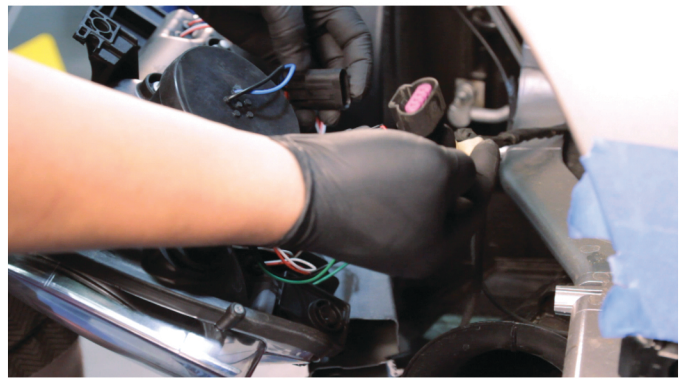
20) Reconnect the low beam harness.
