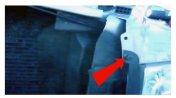
3) Remove the single phillips head screw securing the headlight weatherstrip to the body.
