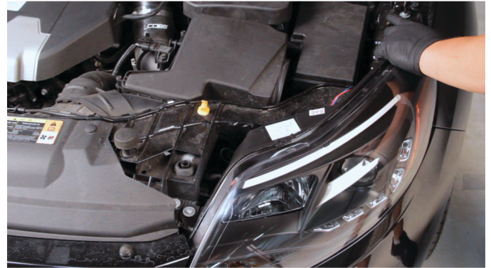
8) Reinstall [2x] T-30 torx screws to secure the headlight.
