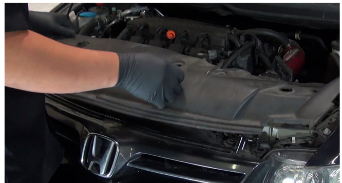
2) After removing retainers, remove Radiator Cover Panel.
