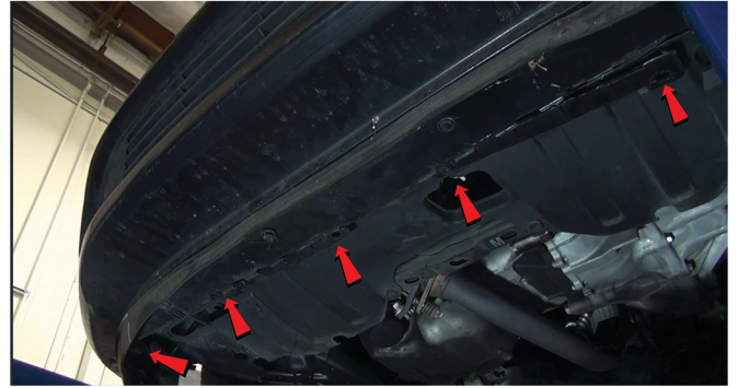
24) Reinstall ten Plastic Retainers Securing Underside of Bumper Fascia
