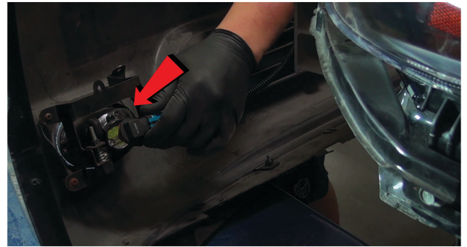
20) Reconnect Fog Light Wiring Harness [if equipped]
