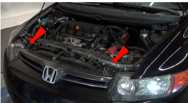
3) Remove two Size 5 Allen Key bolts securing upper bumper fascia.
