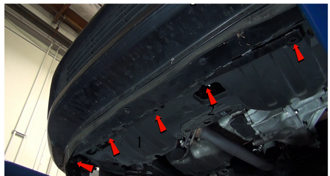
4) Remove ten Plastic Retainers Securing Underside of Front Bumper Fascia to body.
