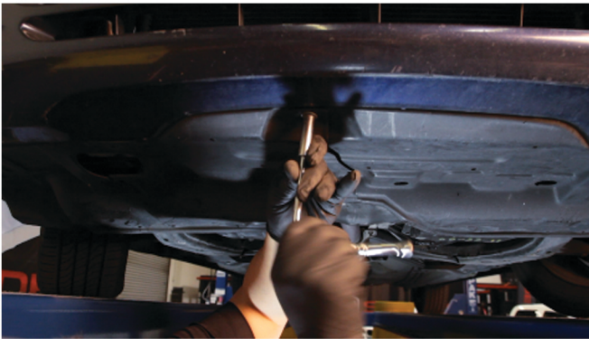
19) Reinstall [7x] 10mm bolts securing the fascia from below.
