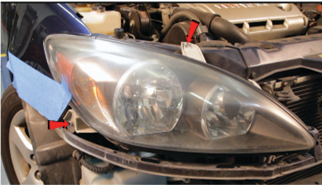
7) Remove [2x] 10mm bolts securing the headlight.
