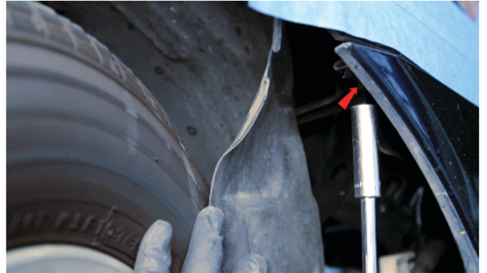
18) Reinstall [1x] 10mm bolt in the fenderwell to secure the front bumper fascia.
