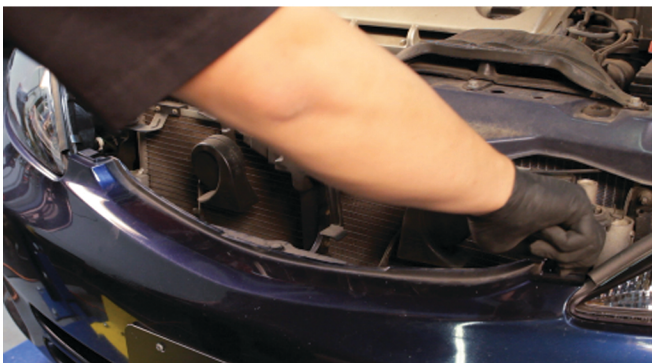
21) Reinstall [2x] 10mm bolts on either side of the grille to secure the fascia.
