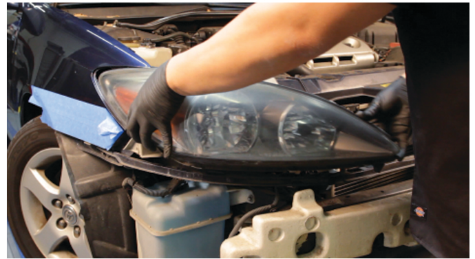
8) Release the headlight retainer tabs, then unseat the headlight.
