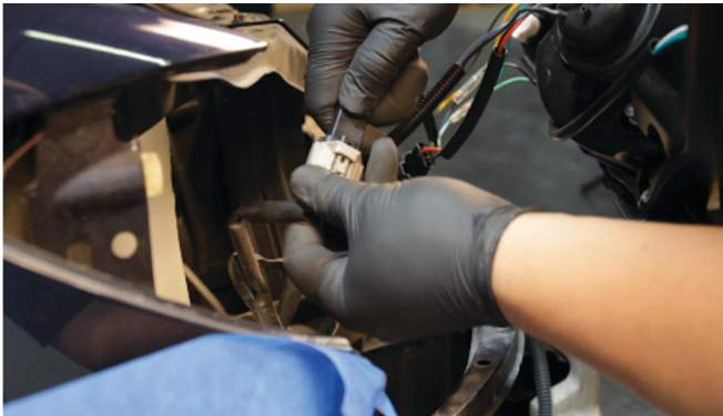
13) Reconnect the turn signal harness.
