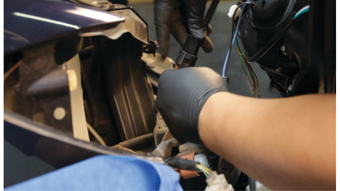
12) Connect the high beam harness to the Spyder headlight.
