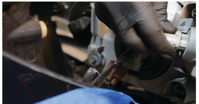
10) Disconnect the turn signal harness.
