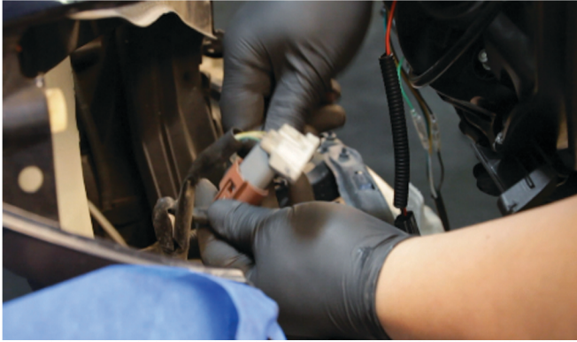
11) Connect the low beam harness to the Spyder headlight.
