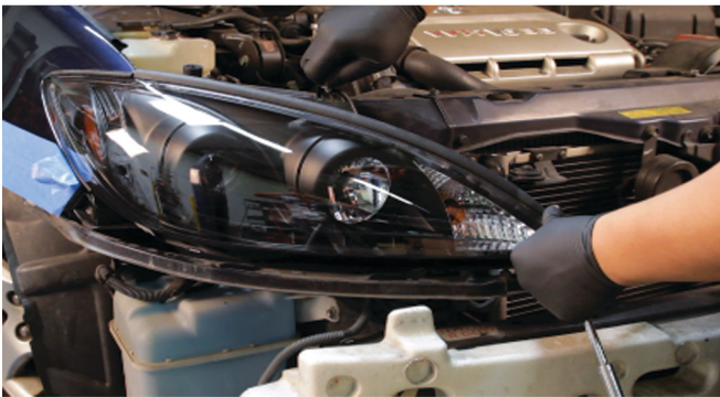
15) Reinstall [2x] 10mm bolts to secure the headlight.
