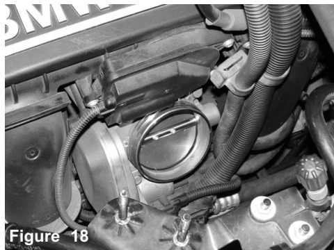
Figure 15 Loosen the throttle body inlet clamp as shown above. The inlet elbow shown above is removed from the 2006 330i
