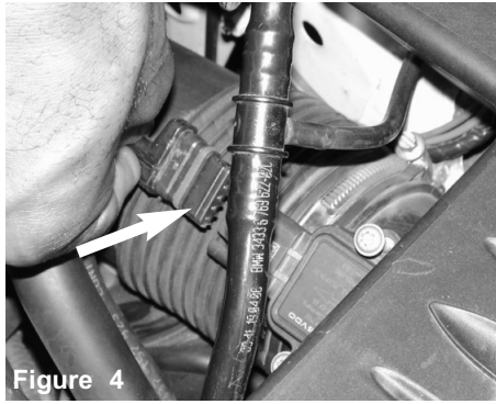
Figure 4 The electrical sensor harness is disconnected.
