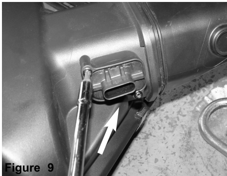
Figure 10 Remove the MAF sensor from the intake tube.
