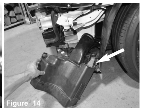
Figure 11 Disconnect the harness that is attached to the base of the air box near throttle body. Now lift up and remove the air box from the vehicle.
