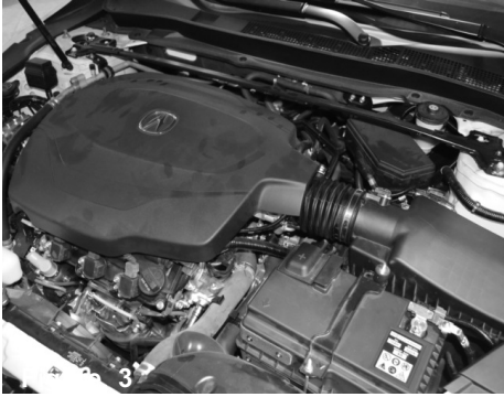
Figure 3 Stock air box shown in this picture, disconnect battery before installation.
