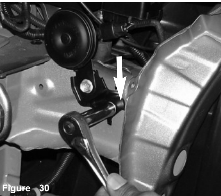
Figure 30 The bolt holding the horn in place is removed. Once the bolt is removed, continue to remove the horn from the stock location.
