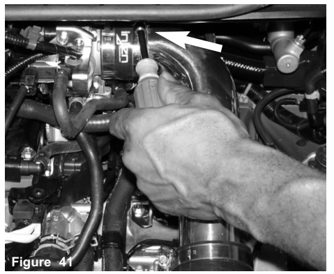
Figure 41 The aluminum and silicone intakes are aligned to each other, once you have aligned the intakes, continue to tighten the throttle body clamp.
