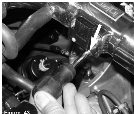
Figure 43 The stock bolts are used to fasten the MAFS to the sensor adapter.
