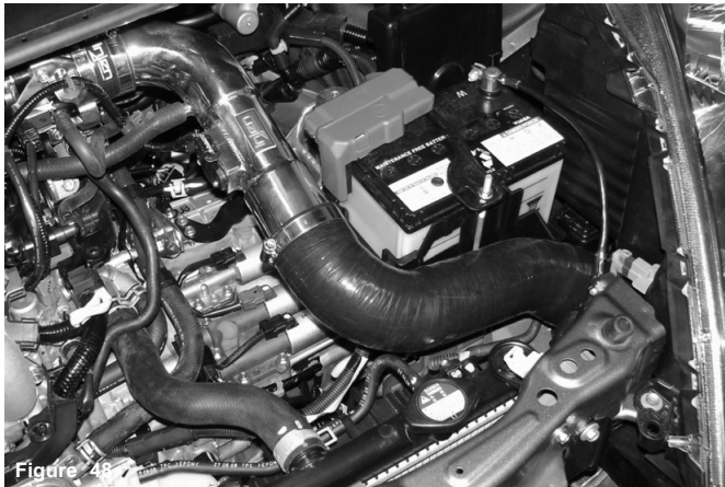
Align the entire intake for the best possible fit. Once the intake has been cleared from all moving parts, continue to tighten all nuts, bolts and clamps. Periodically, check the fitment of the entire intake to prevent damage to the intake. Figure 48
