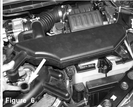
Figure 6 Pull the air resonator box from the side stand-off and remove the resonator box.
