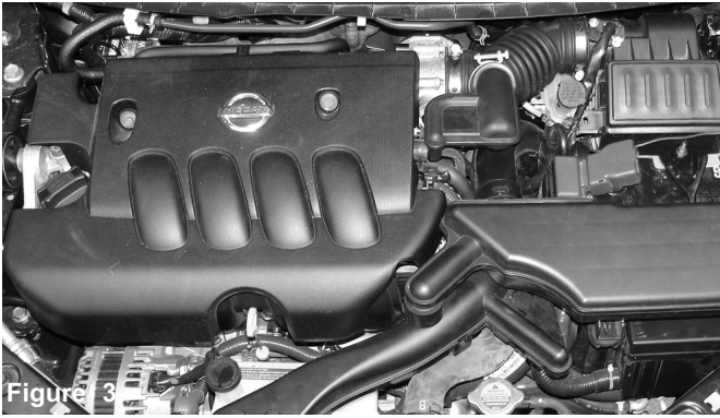
Figure 3 Prior to starting the installation, remove the 2 m6 bolts holding the engine cover in place
