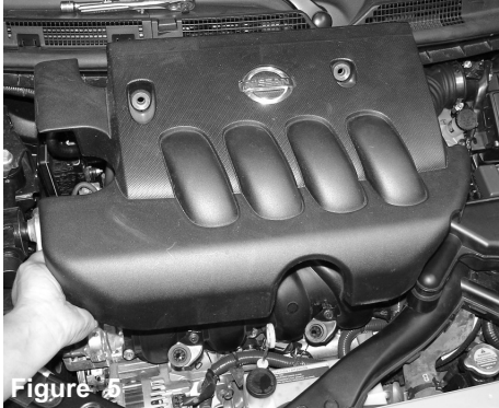
Figure 5 Once you have removed both bolts, continue to pull the engine cover off.
