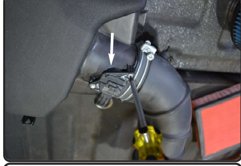
9. Loosen the 2 screws holding in the MAF sensor using phillips screwdriver. Carefully remove the MAF sensor out of the vehicle.
