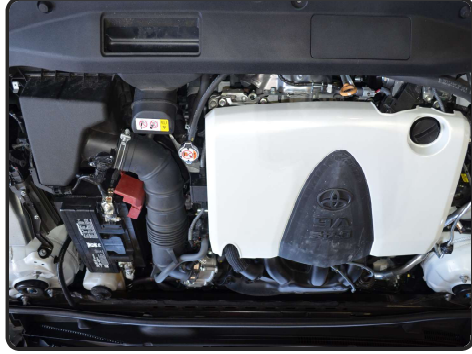
1. Stock intake system shown.
