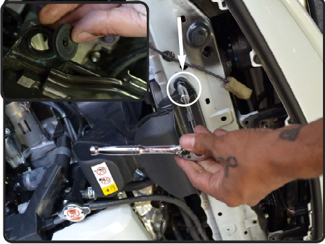
13. Loosen the 1 bolt holding in the OEM Ram scoop. This is where the heatshield will mount to. Remove the 1 grommet from the oem air box mounting brackets.
