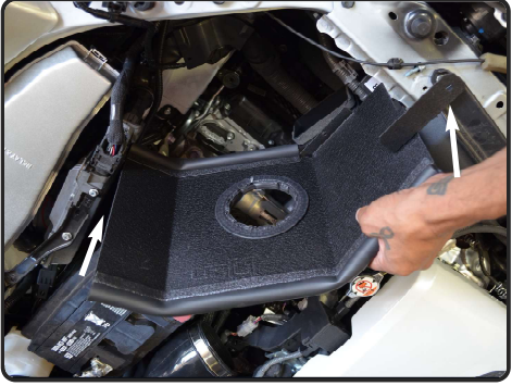
14. Now install the heatshield and position the brackets on heatshield to other mounting points.
