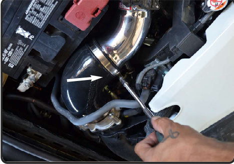
26. Adjust for fitment, tighten all clamps using 8mm nut driver.
