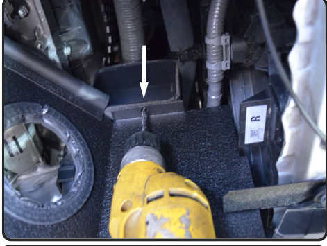
14. Now install the heatshield and position the brackets on heatshield to other mounting points.
