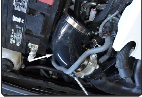
18. Drill hole to 1/4" on the OEM ram scoop.
