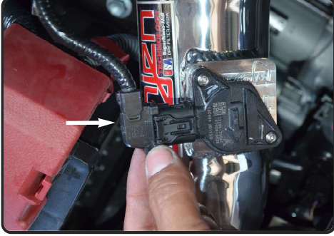
29. Re-connect the MAF sensor harness. Re-install the radiator plastic cover and secure.
