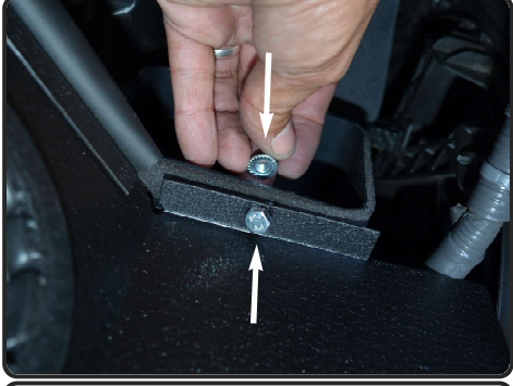
15. Secure the back of heatshield using M6 screw and M6 nut and washer. Make sure Fender washer is secure on the nut side.
