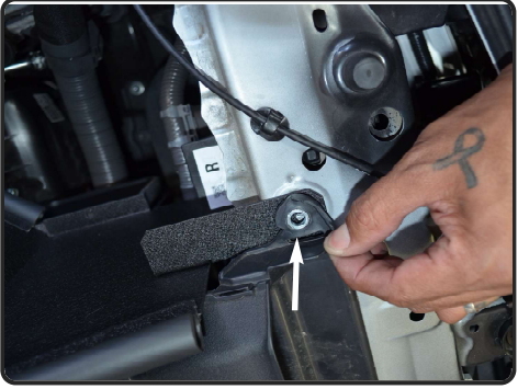
16. Place the tab under the ram scoop and tighten using OEM screw. Secure and tighten.
