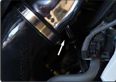
27. Secure the crankcase line to the 5/8" fitting on intake tube and secure using OEM clamp.
