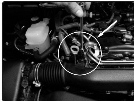
5. Loosen the bolt holding in the stock intake tube using 10mm socket or wrench.
