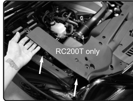
7. RC200T remove the plastic push clips, remove the side engine cover.
