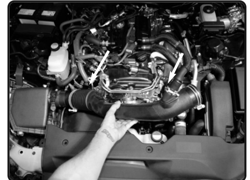
7. Lift up and remove the intake tube from vehicle.
