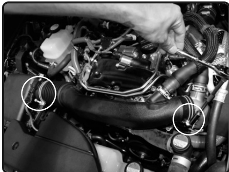
4. Loosen the 2 clamps on the intake tube using 10mm socket or wrench.
