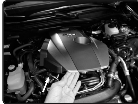
2. Lift up and remove the engine cover.
