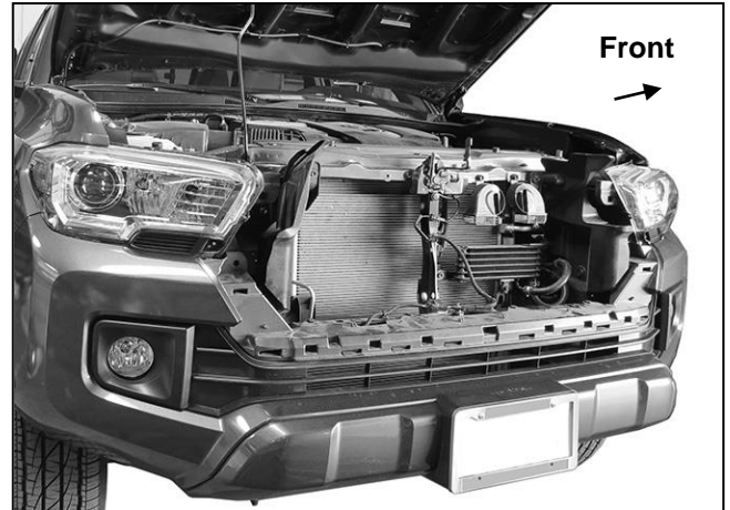
(Fig 11) Grille Removed. Remove factory bumper bolts along the top and bottom of bumper cover
