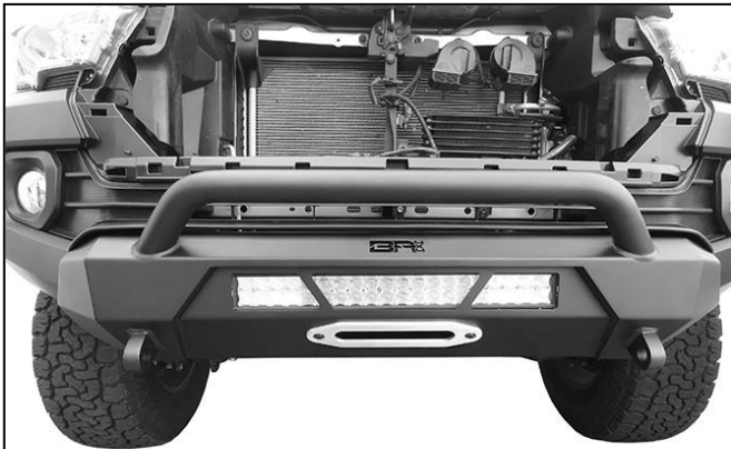
(Fig 29) Check fit of Bumper to plastic and trim as necessary. Reinstall grille and top cover
