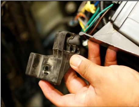
Separate lower headlight mount from factory headlight and set aside.
