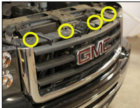
Remove four 10mm bolts from top of radiator grill.
