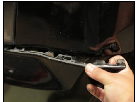
Pull front fascia outward and forward to unclip from fender. Repeat on opposite side.
