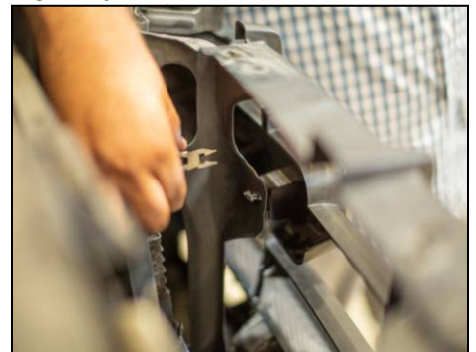
Use needle nose pliers to release both clips from radiator grill. Remove grill and set aside.
