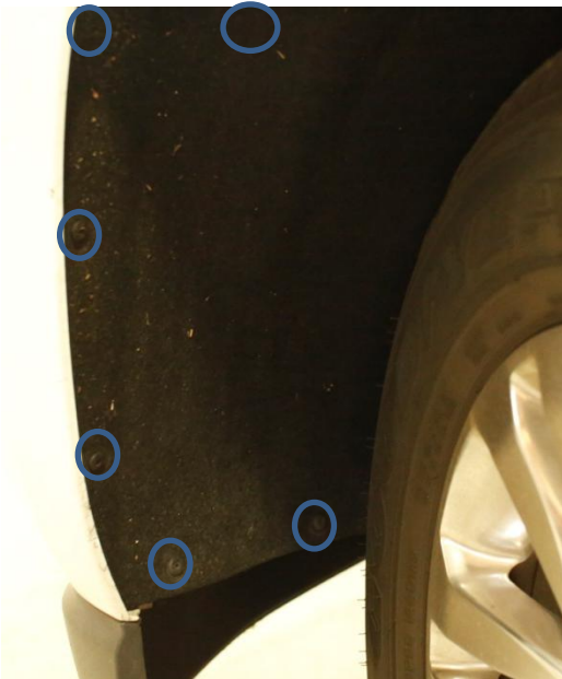
Step 5: Remove six T15 Torx bit screws to peel back tire shroud, within bumper you will locate three 7mm bolts that must be removed.
