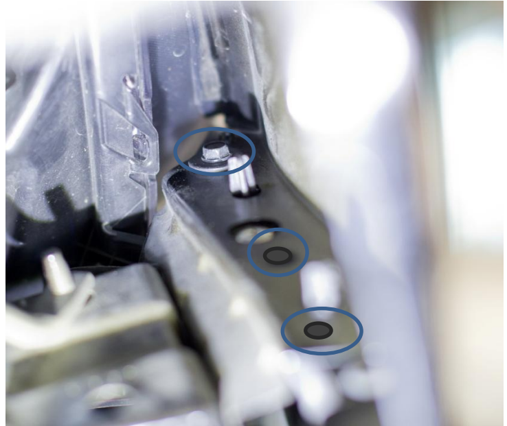
Step 5B: Picture of the inside of the bumper and removing of the three 7mm bolts, repeat step 5 on passenger side.
