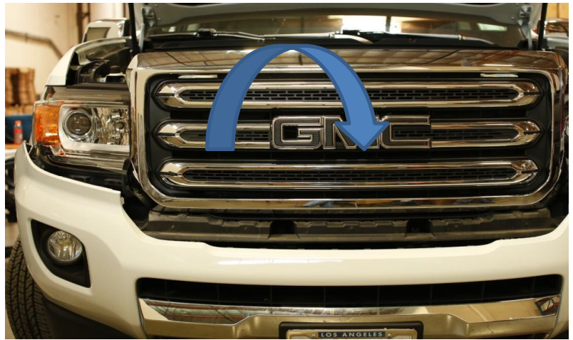
Step 9: With the front bumper being fully detached from grill, you can gently detach the grill from the truck. Tip: Once you detach the grill from each headlight, lean the grill forward and pull out.
