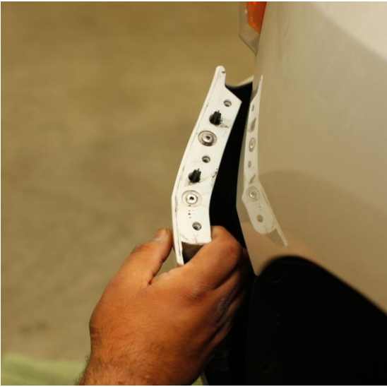
Step 6: Gently pull down on the side of the bumper to detach from fender, repeat process on passenger side.
