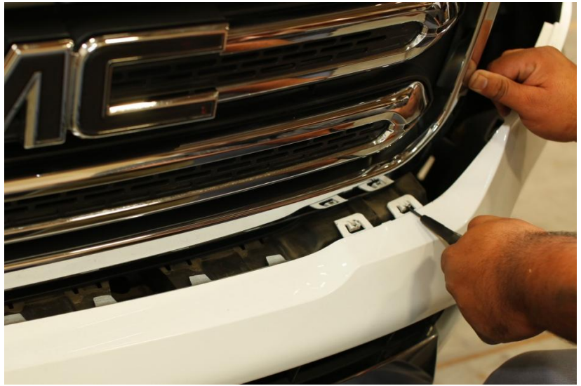
Step 7: Detach two clips from under grill with panel popper or small flat head screwdriver, repeat process on passenger side.
