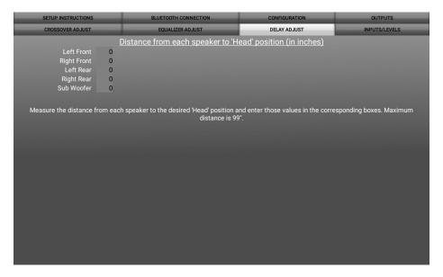
• Allows a delay of each channel. If a delay is desired, first measure the distance (in inches) from each speaker to the listening position, then enter those values to the corresponding speaker. Add (in inches) to the desired speaker to delay it.
