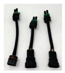
5. Plug the adapter into the OEM plug. Some vehicle kits will come with the adapter unpinned and require that you check polarity of the plug leads. Using a multimeter or circuit tester, determine which wire is the ground (-) and which is positive (+12V-14V). The positive wire will correspond to the Weather pak (Baja Designs plug) terminal location B. Attach the weather pak on the end of the harness so it connects to positive voltage.
