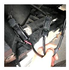
6. Plug in the other two leads to the two lights and secure the harness out of the way. You are now ready to use your fog lamps that will be activated by the factory switch!
