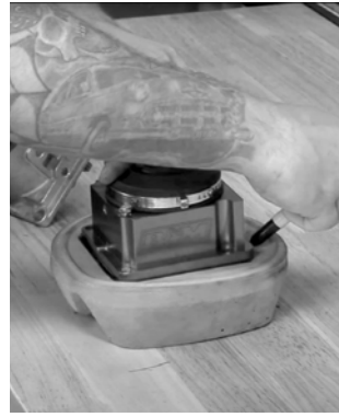
34. Trace the shifter's outline onto the seal. Then remove the shifter, and draw another square inside the first, about 1/4" smaller all around.
