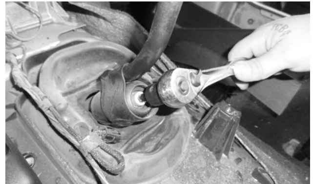
14. Reinstall the floor pan cover, tucking the rear half of its left side under the transfer case shifter flange. Then install the shift lever on the shifter.
