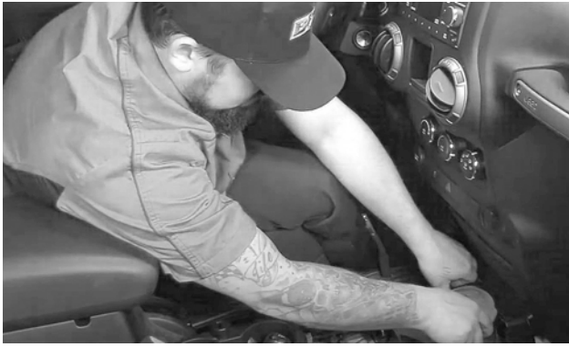
31. Inside the vehicle, remove the seal from around the shifter.
