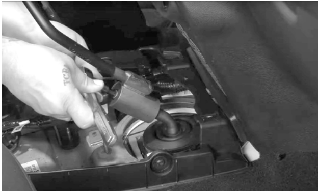
44. Inside the vehicle, reinstall the shift lever on the B&M shifter with the stock screw.
