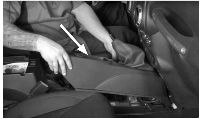
46. With both the transmission and transfer case shifters in NEUTRAL , reinstall the center console.
