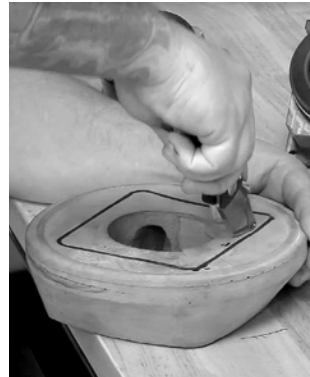
35. Carefully cut through the seal along the inner line, to allow the B&M shifter to fit snugly inside the seal.
