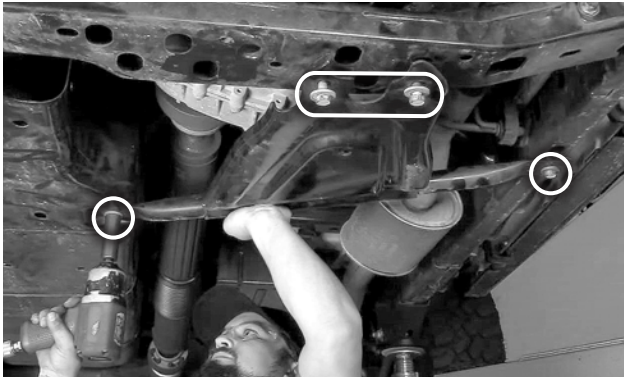
43. Reinstall the transfer case skid plate.
