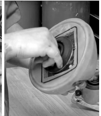
35. Carefully cut through the seal along the inner line, to allow the B&M shifter to fit snugly inside the seal.
