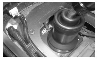
15. Install the vent hose on the fitting on the front of the shifter.
