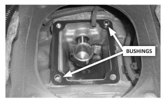
12. If either of the 2 alignment bushings, or the gasket, remains with the shifter, return them to their locations on the shifter mount pad.
