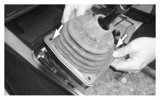
21. Lower the rest of the cover plate assembly over the shift lever, carefully working the boot's opening around the screw heads on the lever.
