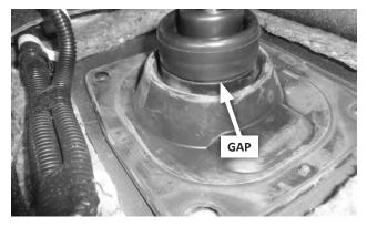
• The top edge of the lower dust boot will sit just below the bottom edge of shifter boot. (There will be a slight gap between them.)
