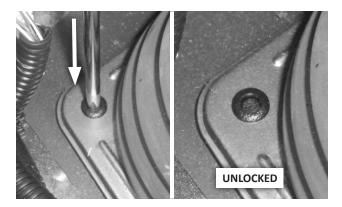
8. Unlock the 2 plastic push rivets at the front of the cover plate by depressing their center plungers slightly (about 1/16") with a punch or small Phillips head screwdriver.
