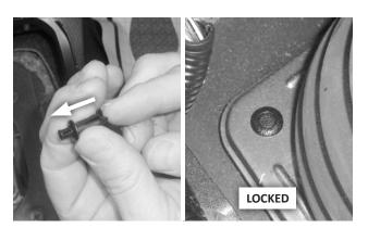
**22. Re-set the plungers on the 2 push-lock fasteners** by pushing them up from the bottom end. Then insert the fasteners in their holes and lock them by pushing the plungers down flush.
