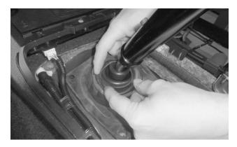
**20.** Install the lower dust boot over the shift lever, and work it down over the rubber boot on the shifter.
