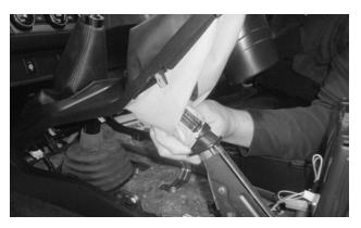
5. While lifting the console panel upward, turn the parking brake boot inside out, and work its elastic opening over the end of the parking brake lever.
