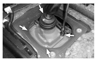
**11. Put the shifter in NEUTRAL.** Remove the 4 mount screws, then remove the stock shifter.
