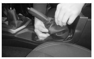
**28.** Work the leather boot down over the parking brake lever, working its elastic opening into the groove on the lever.
