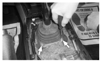
7. Remove the 2 screws at the rear of the cover plate assembly.
