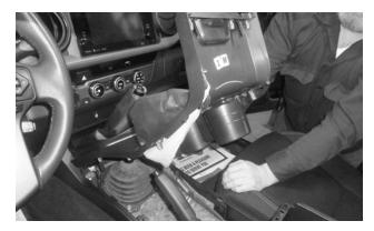
6. When the parking brake boot is clear of the lever, remove the console trim panel and set it aside.
