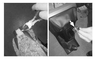
24. On the upper console panel, turn the leather boot insideout, cut the cable tie, and remove the chrome trim ring.
