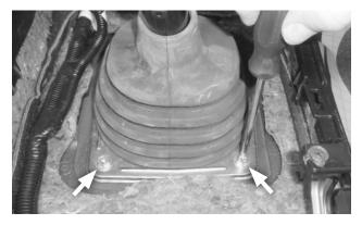
23. Re-install the 2 cover plate screws.
