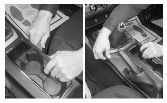
**4.** Use a plastic trim removal tool to separate the upper console panel from the console base.
