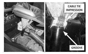
**25.** With the leather boot still turned inside-out, work its opening down over the shift lever until the impression from the old cable tie is located over the groove on the lever.
