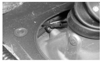
**10. Carefully remove the rubber vent hose from the barb fitting** on the front of the shifter housing.
