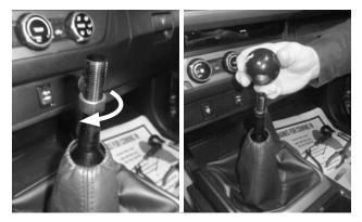
**30.** Run the jam nut all the way down the threads, then install the shift knob.
