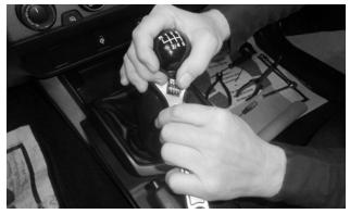
**31.** Turn the knob all the way down until it touches the nut. Then back it off to align it as desired, and tighten the jam nut.
