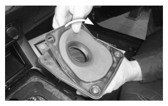
**19. Carefully peel the lower dust boot** off the cover plate assembly.
