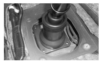
**14. Install the shifter on the mount pad.** First insert the pivot bushing into the shift linkage. Then align the 2 mount pad bushings.
