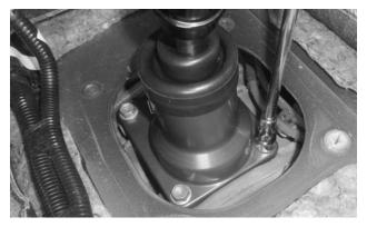
**16. Re-install the stock shifter screws,** and tighten to 13 ft-lbs torque.
