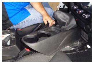
3. Carefully lift the center console cover straight up to disengage it from the console, then remove the cover.
