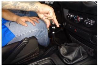
9. With its wrench flats facing down, run the lock nut (2) all the way down the shifter threads. Then run the shift knob (1) as far down the threads as it will go while keeping the B&M logo aligned as desired. Finally, secure the shift knob with the lock nut.
