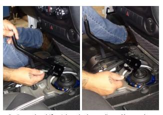
Press the shift stick and adapter (item 3) onto the vehicle's shift lever and secure with the original bolt, then tighten the two set screws on the side of the adapter.
