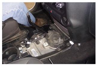
7. Reinstall the shifter boot, then carefully press the sheet metal nut plate onto the stud.
