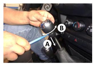
2. Use a trim tool to separate the trim ring from the bottom of the gearshift knob (A). Remove the knob by grasping it firmly with both hands and rotating it back and forth slightly (B) while sharply pulling it straight up. Finally, remove the trim ring from the shift lever. Repeat to remove the shift knob and trim ring from the transfer case.
