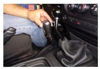
10. Reinstall the trim ring and shift knob on the transfer case shift lever, then snap the trim ring to the bottom of the knob to secure it to the lever.
