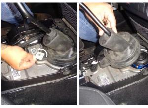
4. <u>CAUTION</u>: The sheet metal nut plate has sharp edges! Carefully remove the sheet metal nut plate, then remove the shifter boot.
