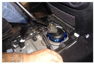
5. Remove the shift stick screw, then pull the shift stick straight off the shift lever.
