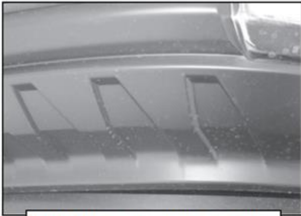
(Fig 4) Temporarily remove the splash guard as required to gain access to the front of the frame channel.
