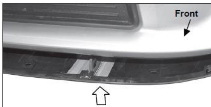
(Fig 9 ) Hold the splash guard up to the bottom of the brackets and mark location for cutting to clear brackets. Cut only what is needed to insert bracket through the splash guard.
