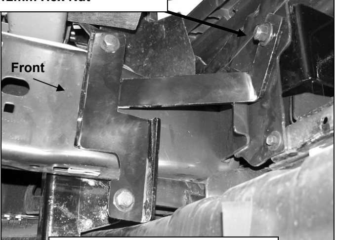
(Fig 8) Inner Support Bracket pictured from behind front bumper
