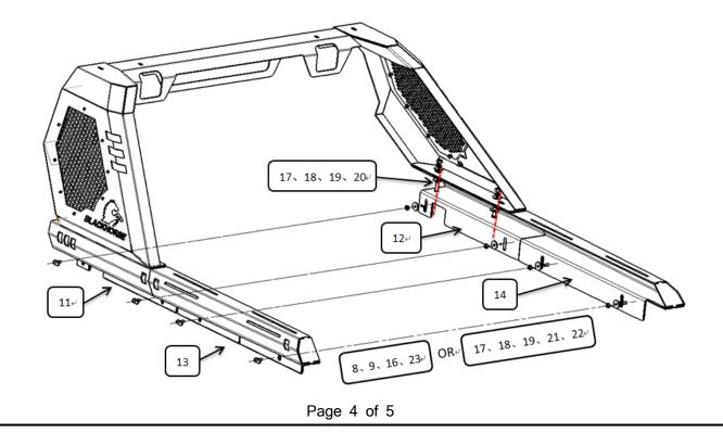
Step 4: Test and make sure that the roll bar is steadily fixed, fully tighten all hardware. Step 5: Installation is finished, pick up all tools.
