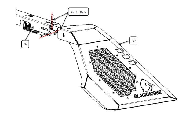
Step 3: Connect brackets and roll bar with standard parts ① 18 19 20 as figure shows. For use without Utility Track in the truck:
